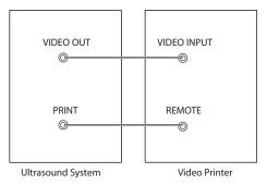
Connect the video printer to the system by BNC cable and Remote Control cable provided by the manufacturer. You can refer the installation method as the above figure shown. The video printer can work without any configurations after a successful connection.
