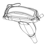
7. Press the handle and insert the biopsy bracket tube into the biopsy bracket.
