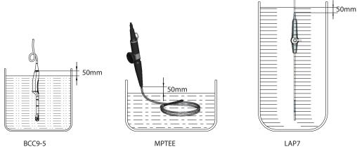
Figure 11-3 Probe Immersion
