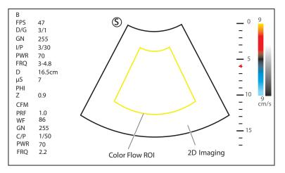
Figure 6-6 CFM-Mode Imaging Screen
