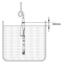
Figure 11-5 Endocavitary Probe Immersion 2
