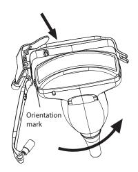
6. Attach the biopsy bracket to the probe and fasten the biopsy bracket with the locking screw.
