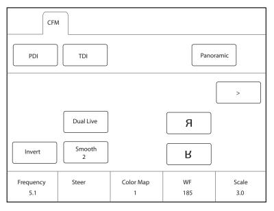
Figure 6-11 CFM/PDI/TDI Mode Imaging Parameters Menu
