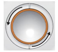
Figure 11-1 Cleaning the Trackball
