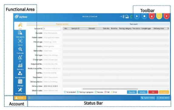
Figure 3-5 Operation interface of software
