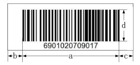
Figure 5-2 Barcode specifications illustration
