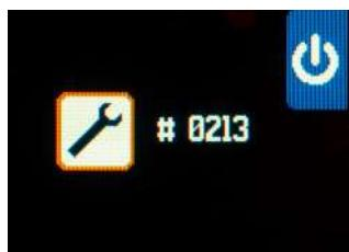
Remove the memory card and re-initialise it with the medilog DARWIN2 Recorder Setup program. If the error remains, proceed as follows:
