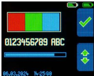
1. Press the LOWER button repeatedly to adjust the Contrast. The test pattern helps to judge the selected contrast setting.
