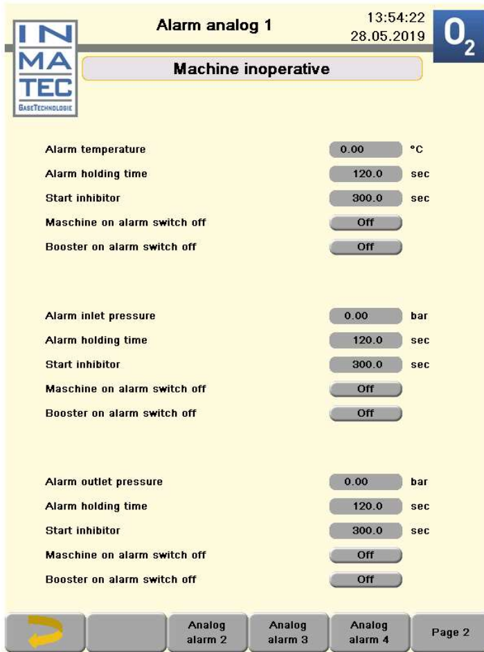
Fig. 11: Alarms control menu: Alarm outlet pressure
