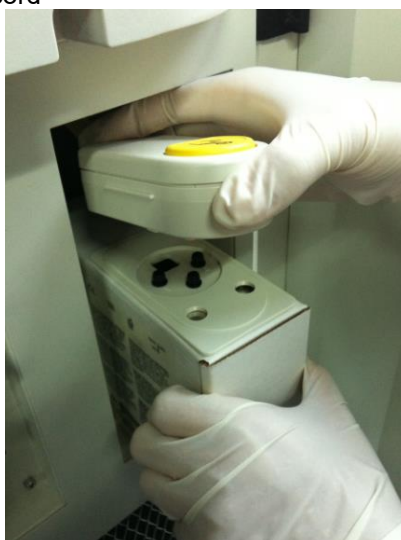
Figure 14-9 ISE reagent pack wand
