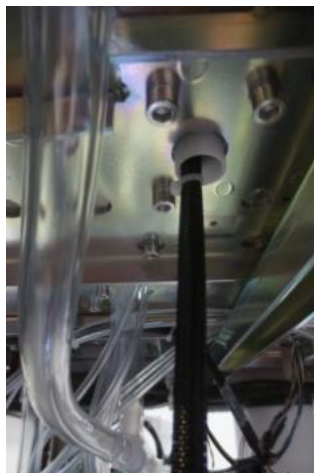
Figure 3-43 Install the braided hose
