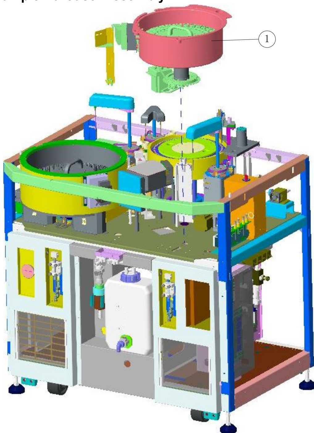
Figure 11-16 Sample carousel assembly
