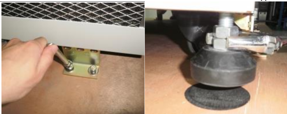
Figure 8-12 Remove the mounting plate, and then screw up the anchors carefully.
