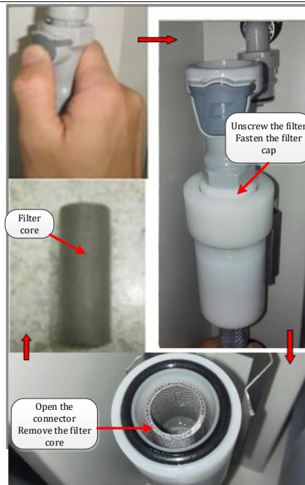
Figure 5-18 Replace the deionized water filter
