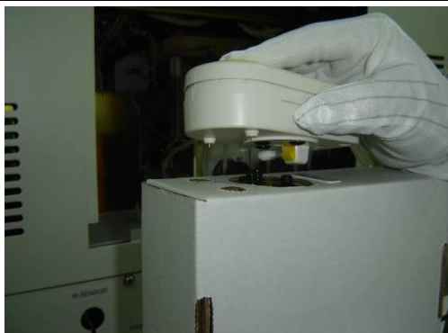
Figure 14-19 Install the reagent pack wand
