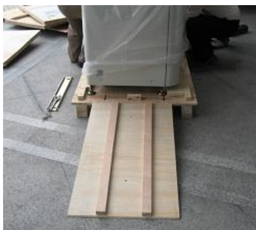
Figure 8-14 Align the slope cover with the analyzer
