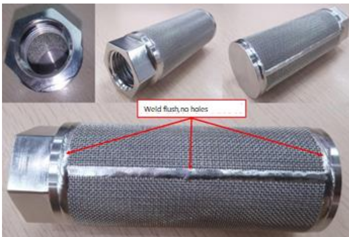
Figure 5-20 Deionized water filter installation
