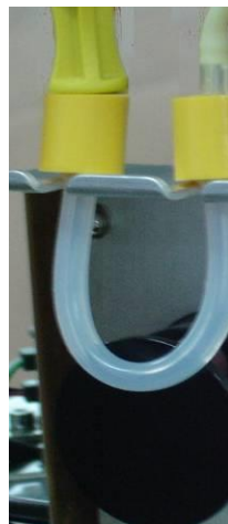
Figure 13-4 Installing Peristaltic Pump Tube
