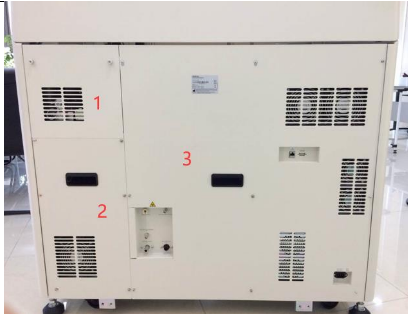
Figure 14-3 Take off the rear panel
