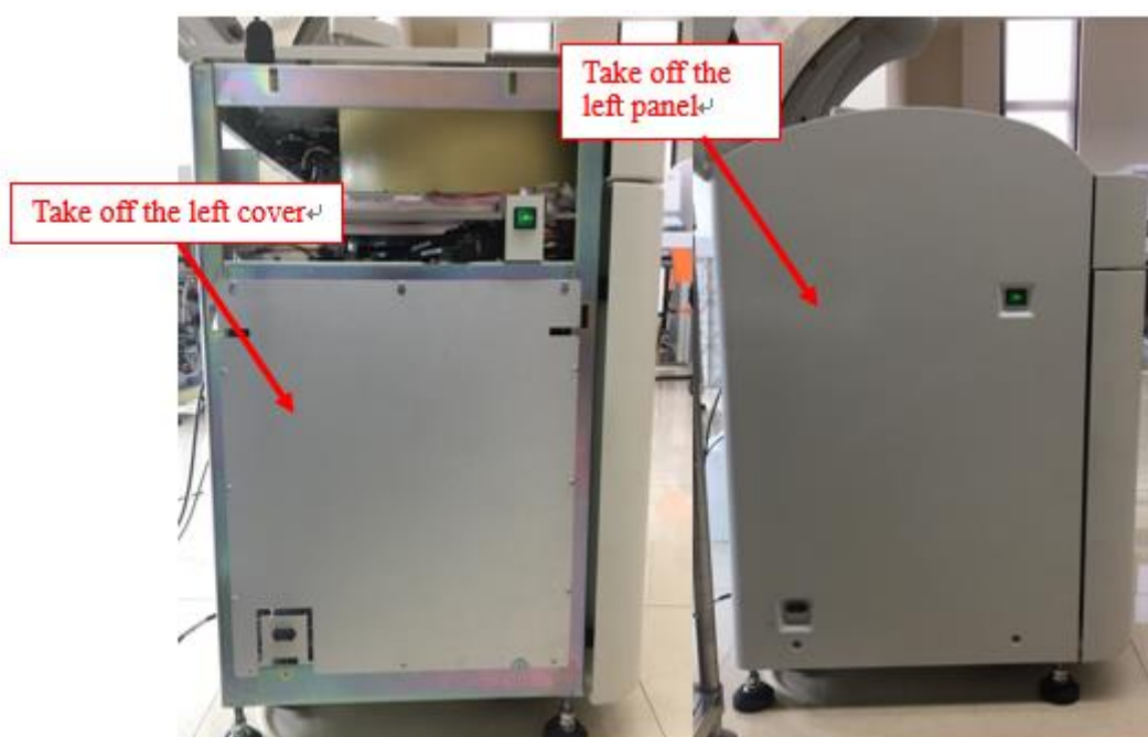
Figure 14-2 Take off the left panel and its baffle
