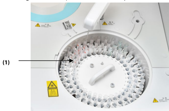
Figure 1.5 Sample carousel assembly
