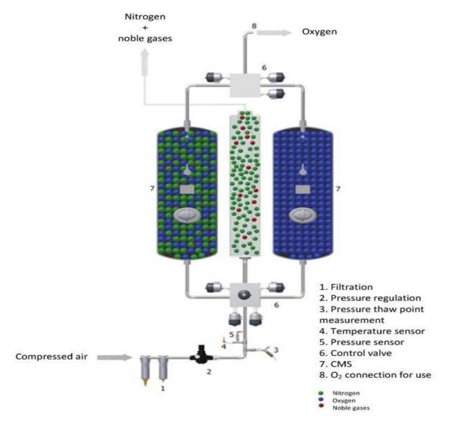
Through the Pressure Swing Adsorption (PSA) technology and adsorption media developed in-house, the atmospheric air is separated in its components nitrogen and oxygen. Subsequently, oxygen is available for further use in quantities of  $0.5 - 2.000,00 \text{ Nm}^3/\text{h}$  and purities of 90.0 - 95%.
