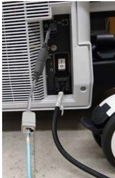
Figure 3-7. LAN cable with protection cable (example)
