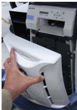
Figure 12-9. Remove the front cover
