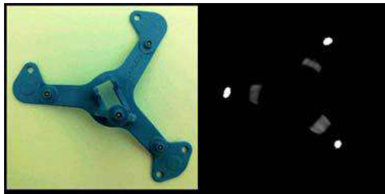
Figure 13-153. Left, Active Tracker - Right, CT of Active Tracker
