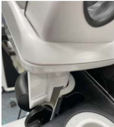
Figure 3-3. Install TVTR Probe holder
