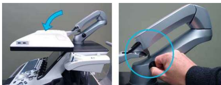
Figure 3-41. Flip down the monitor and lock the monitor arm
