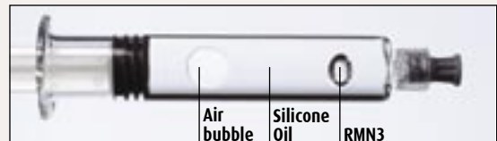
Syringe stored for 5 days at +5°C. Solution is separated and cannot be used.
