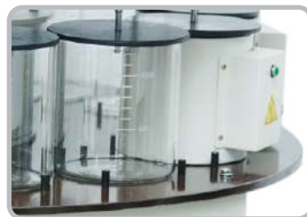
Wax bath with over heat protection for tissue safety
