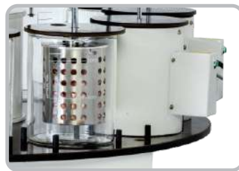
Wax Bath with over heat protection
