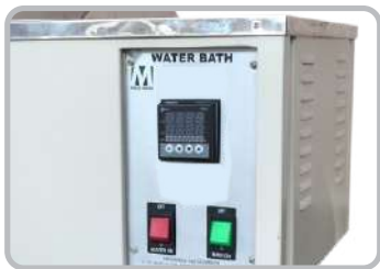
PID/Analog Control Panel
