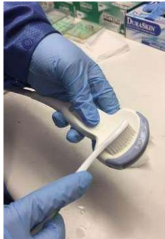
Figure 11-6. Cleaning the probe using a brush
