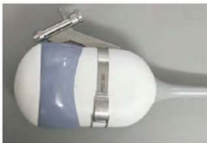
Figure 11-44. Mounting the Biopsy Needle Guide to the 4D Probe
