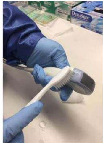
Figure 11-6. Cleaning the probe using a brush
