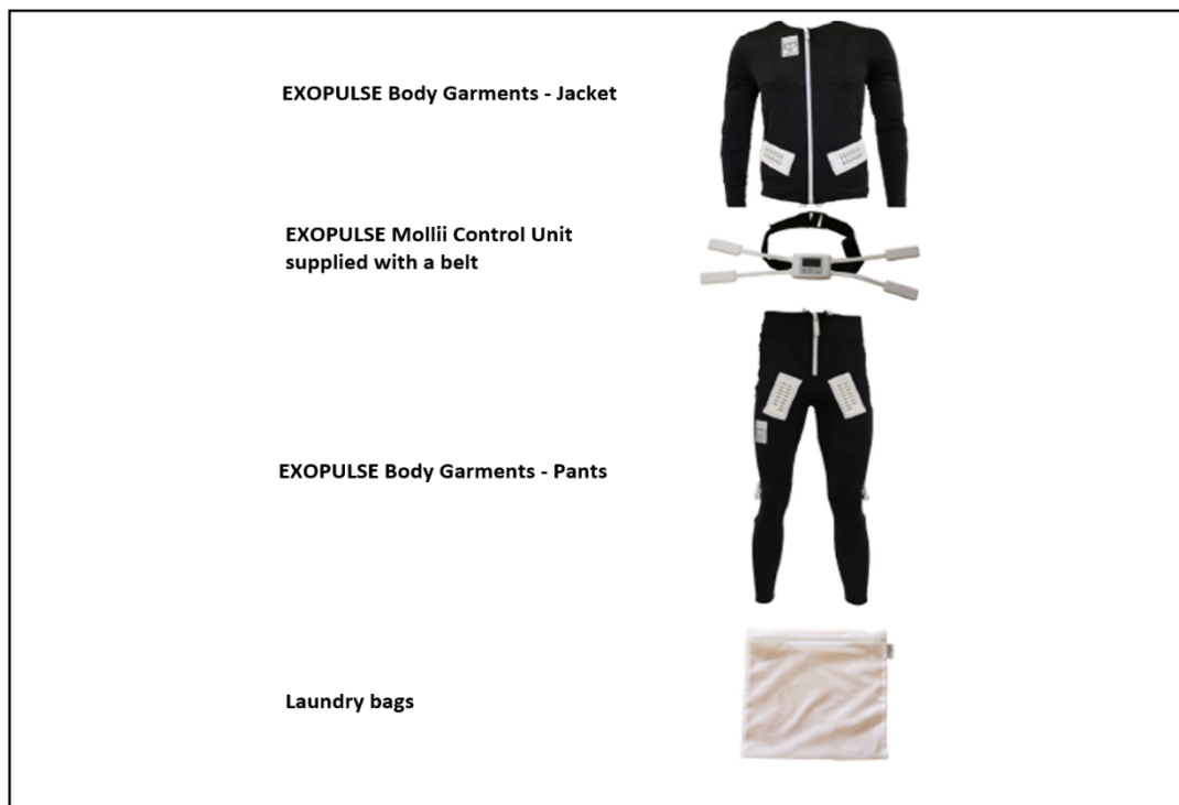
Figure 1. Overview of the EXOPULSE Mollii Suit. The EXOPULSE Mollii Suit consists of garments (jacket and pants) with embedded electrodes, a detachable EXOPULSE Mollii Control Unit and laundry bags. The figure is adapted from IFU EXOPULSE Mollii Suit .
