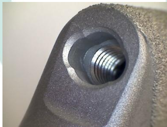
FIG.8: THREADED HOLE FOR INSERTION INSTRUMENT
