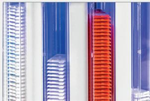
The number of remaining cassettes can be easily seen through the transparent loading chutes with blue LED backlight.
