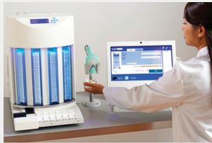
The Autoloader version in combination with the Printtec C has been specially designed for fast and efficient processing. The magazines with the cassettes are simply inserted into the loading chutes.
