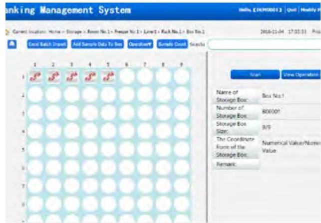
2. The Crown visual interface displays a visual representation of every level of a lab's sample storage from freezers to individual samples, allowing users to review their sample storage status at a glance.
