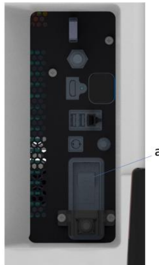
Figure 1-40. Circuit Breaker (located on the rear panel)
