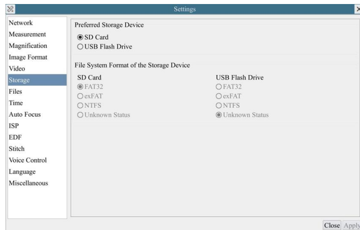
Figure 34 Comprehensive Setting of Storage Page
