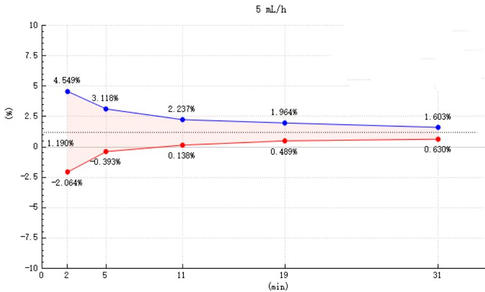
**Graph 8 Trumpet curve: Percentage variation Ep against observation window duration P (min) and the overall mean percentage error A plotted from data gathered during the second hour of the test period.**
