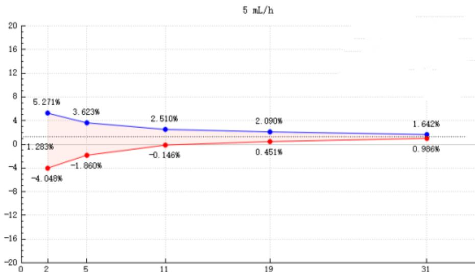
**Graph 4 Trumpet curve: Percentage variation  $E_p$  against observation window duration P (min) and the overall mean percentage error A plotted from data gathered during the second hour of the test period.**
