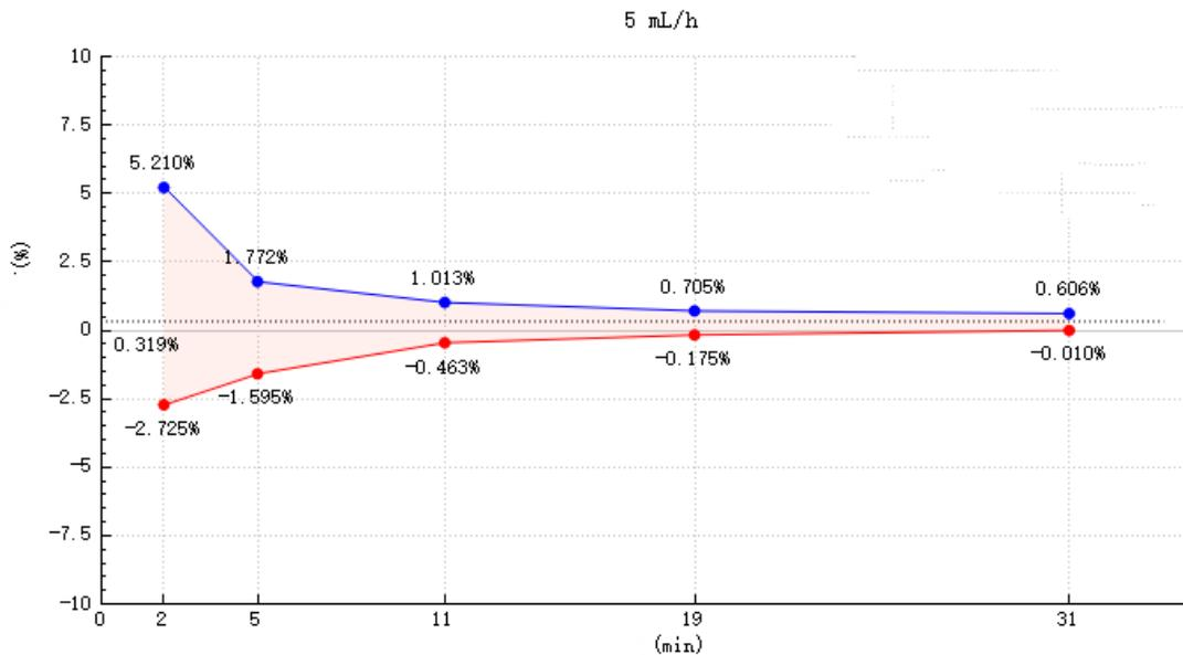
**Graph 6 Trumpet curve: Percentage variation  $E_p$  against observation window duration P (min) and the overall mean percentage error A plotted from data gathered during the second hour of the test period.**
