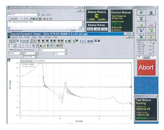
Recordings of signals from control sensor and sensor recording the vibration responses, cable ladder type A 20–FM–100–15, at test of seismic eligibility Level S2 there in "x" axis.
