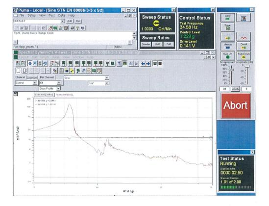
Recordings of signals from control sensor and sensor recording the vibration responses, cable ladder type A 20–FM–100–15, at test of resonant frequency assessment there in "z" axis.
