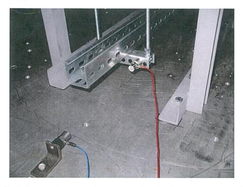
Location of both the control sensor and sensor recording the vibration responses while testing the cable trays type A 05–05A–15 there in "z" axis.
