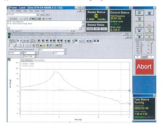
Recordings of signals from control sensor and sensor recording the vibration responses, cable trays type A 05–05A–15, at test of resonant frequency assessment there in "y" axis.
