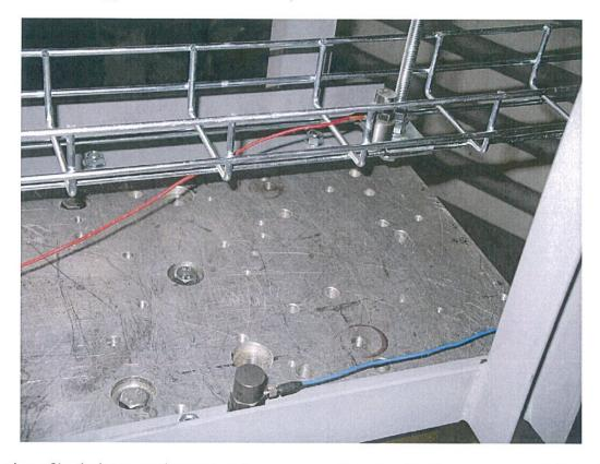
Location of both the control sensor and sensor recording the vibration responses while testing the cable channel type ATK-10-15 there in "x" axis.
