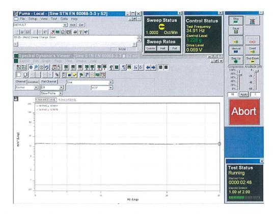
Recordings of signals from control sensor and sensor recording the vibration responses, cable channel type ATK-10-15, at test of resonant frequency assessment there in "x" axis.
