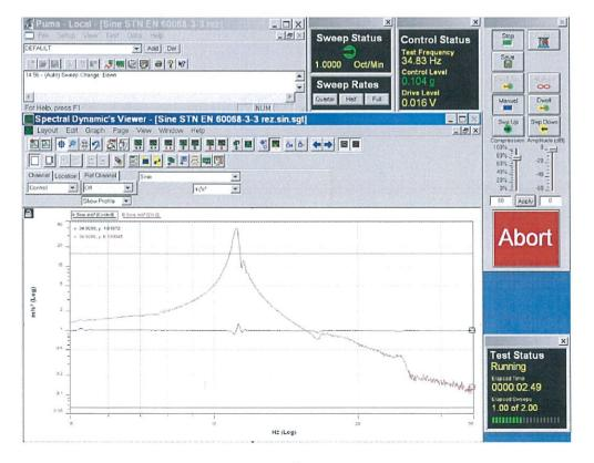
Recordings of signals from control sensor and sensor recording the vibration responses, cable channel type ATK-10-15, at test of seismic eligibility Level S1 there in "x" axis.
