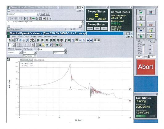
Recordings of signals from control sensor and sensor recording the vibration responses, cable trays type A 05–05A–15, at test of seismic eligibility Level S2 there in "x" axis.
