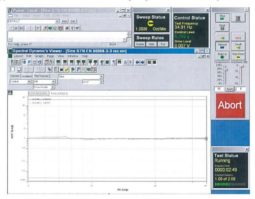
Recordings of signals from control sensor and sensor recording the vibration responses, cable trays type A 05–05A–15, at test of seismic eligibility Level S1 there in "y" axis.
