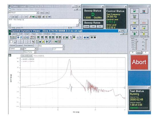
Recordings of signals from control sensor and sensor recording the vibration responses, cable trays type A 05–05A–15, at test of seismic eligibility Level S1 there in "x" axis.
