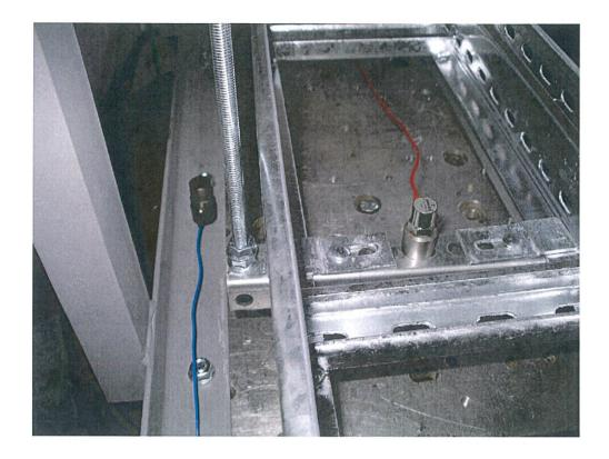
Location of both the control sensor and sensor recording the vibration responses while testing the cable ladder type A 20–FM–100–15 there in "x" axis.
