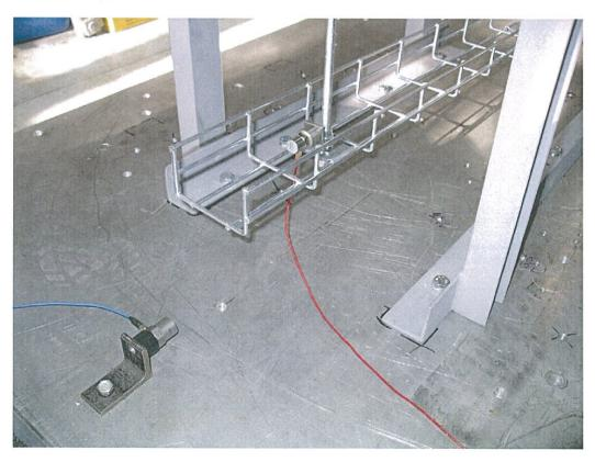
Location of both the control sensor and sensor recording the vibration responses while testing the cable channel type ATK-10-15 there in "z" axis.
