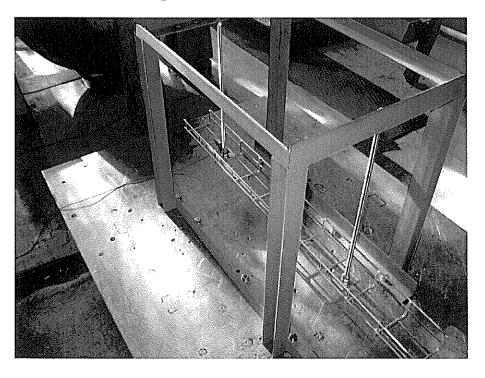
Fixing the testing assembly of cable ladder type A 20–FM-100–15 in testing apparatus and its "z" axis orientation thereto on vibrating stand
