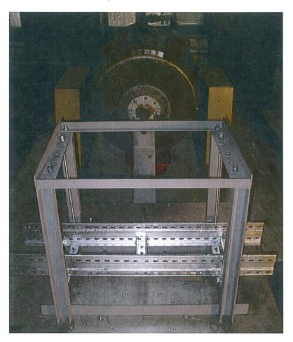
Fixing the testing assembly of cable trays type A 05-05A-15 in testing apparatus and its "z" axis orientation thereto on vibrating stand
