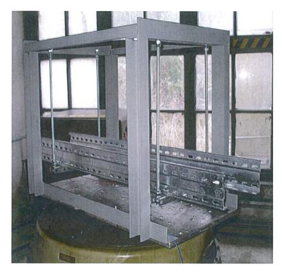
Fixing the testing assembly of cable trays type A 05-05A-15 in testing apparatus and its "y" axis orientation thereto on vibrating stand
