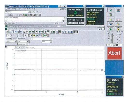
Recordings of signals from control sensor and sensor recording the vibration responses, cable channel type ATK-10-15, at test of seismic eligibility Level S1 there in "y" axis.
