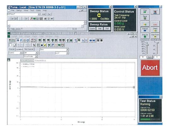
Recordings of signals from control sensor and sensor recording the vibration responses, cable trays type A 05–05A–15, at test of seismic eligibility Level S2 there in "y" axis.
