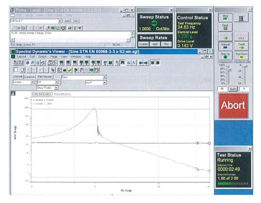
Recordings of signals from control sensor and sensor recording the vibration responses, cable channel type ATK-10-15, at test of resonant frequency assessment there in "z" axis.
