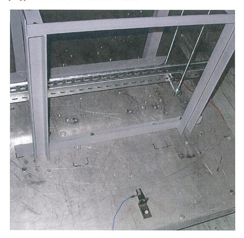
Location of both the control sensor and sensor recording the vibration responses while testing the cable channel type ATK-10-15 there in "y" axis.
