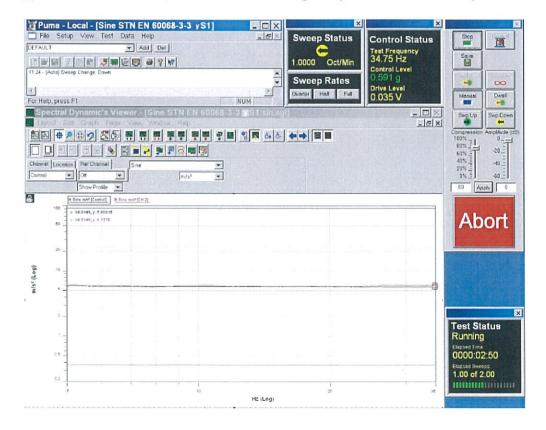
Recordings of signals from control sensor and sensor recording the vibration responses, cable ladder type A 20–FM–100–15, at test of seismic eligibility Level S2 there in "y" axis.
