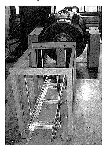
Fixing the testing assembly of cable trays type A 05-05A-15 in testing apparatus and its "x" axis orientation thereto on vibrating stand
