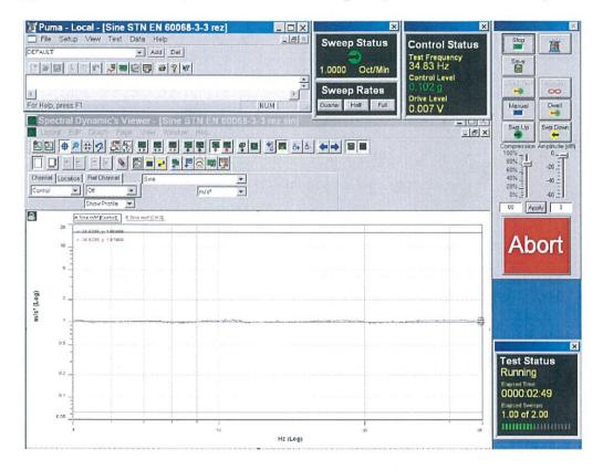
Recordings of signals from control sensor and sensor recording the vibration responses, cable ladder type A 20–FM–100–15, at test of seismic eligibility Level S1 there in "y" axis.
