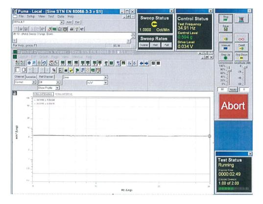
Recordings of signals from control sensor and sensor recording the vibration responses, cable channel type ATK-10-15, at test of seismic eligibility Level S2 there in "y" axis.
