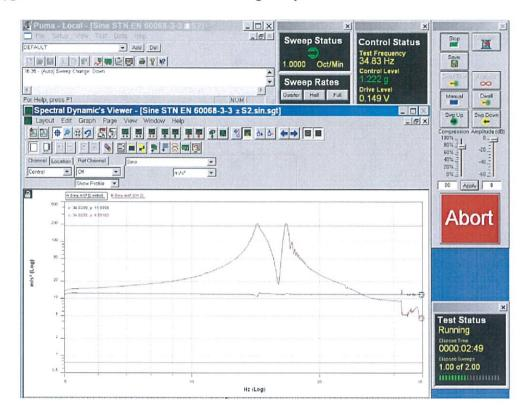
Recordings of signals from control sensor and sensor recording the vibration responses, cable channel type ATK-10-15, at test of resonant frequency assessment there in "y" axis.
