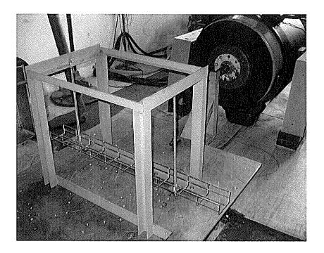
Location of both the control sensor and sensor recording the vibration responses while testing the cable ladder type A 20–FM–100–15 there in "y" axis.
