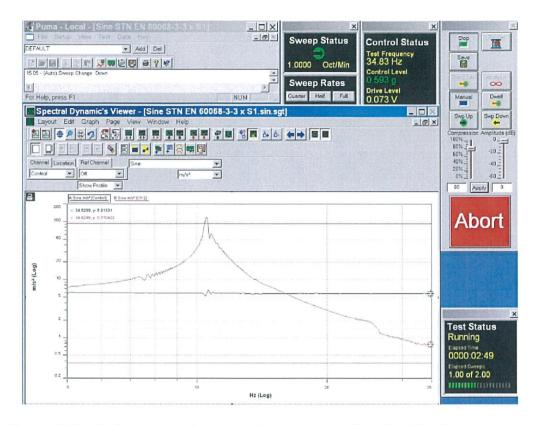
Recordings of signals from control sensor and sensor recording the vibration responses, cable channel type ATK-10-15, at test of seismic eligibility Level S2 there in "x" axis.
