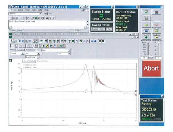
Recordings of signals from control sensor and sensor recording the vibration responses, cable trays type A 05–05A–15, at test of seismic eligibility Level S2 there in "z" axis.
