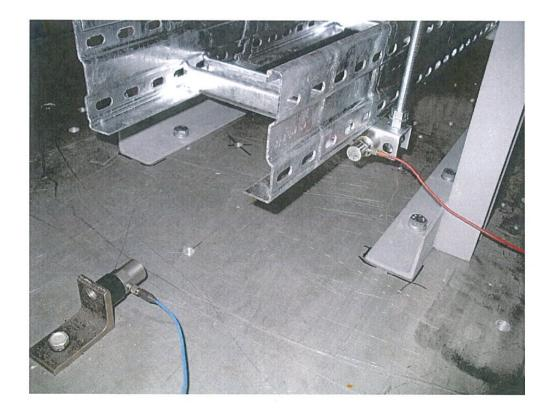
Location of both the control sensor and sensor recording the vibration responses while testing the cable ladder type A 20–FM–100–15 there in "z" axis.
