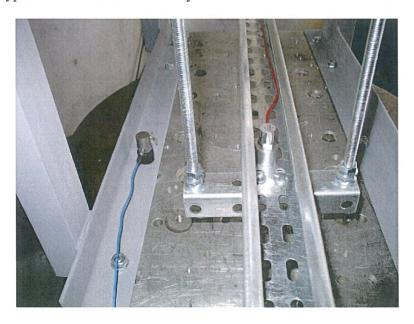
Location of both the control sensor and sensor recording the vibration responses while testing the cable trays type A 05-05A-15 there in "x" axis.
