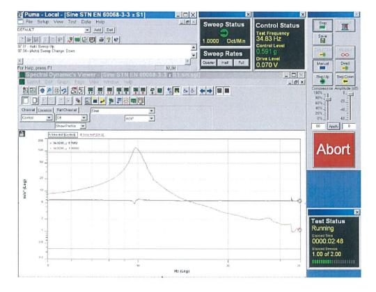
Recordings of signals from control sensor and sensor recording the vibration responses, cable ladder type A 20–FM–100–15, at test of seismic eligibility Level S2 there in "z" axis.
