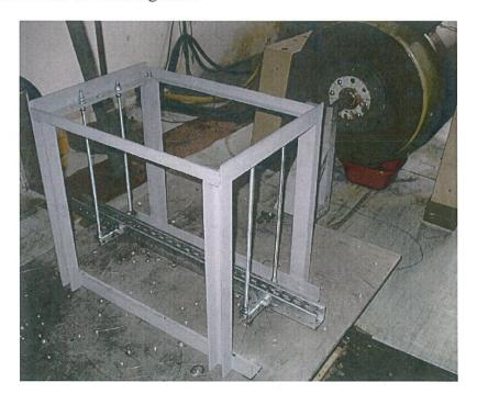
Fixing the testing assembly of cable channel type ATK-10-15 in testing apparatus and its "z" axis orientation thereto on vibrating stand
