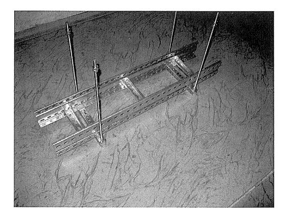
Testing assembly of cable trays type A 05–05A–15
