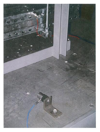
Location of both the control sensor and sensor recording the vibration responses while testing the cable trays type A 05–05A–15 there in "y" axis.
