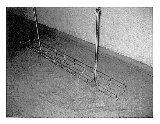
Fixing the testing assembly of cable ladder type A 20-FM-100-15 in testing apparatus and its "y" axis orientation thereto on vibrating stand
