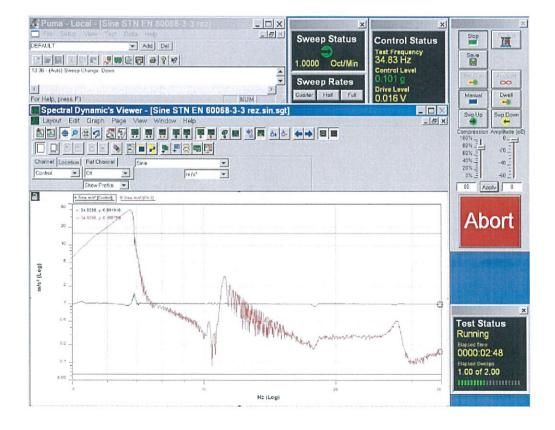
Recordings of signals from control sensor and sensor recording the vibration responses, cable ladder type A 20–FM–100–15, at test of seismic eligibility Level S1 there in "x" axis.
