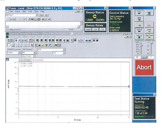
Recordings of signals from control sensor and sensor recording the vibration responses, cable trays type A 05–05A–15, at test of resonant frequency assessment there in "x" axis.
