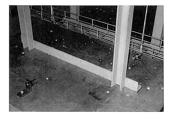
Recordings of signals from control sensor and sensor recording the vibration responses, cable ladder type A 20–FM–100–15, at test of resonant frequency assessment there in "y" axis.
