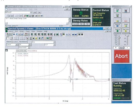
Recordings of signals from control sensor and sensor recording the vibration responses, cable trays type A 05–05A–15, at test of seismic eligibility Level S1 there in "z" axis.
