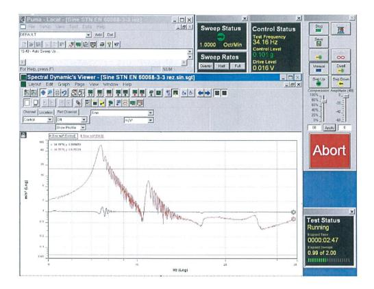
Recordings of signals from control sensor and sensor recording the vibration responses, cable channel type ATK-10-15, at test of seismic eligibility Level S1 there in "z" axis.
