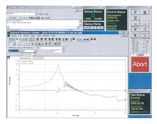
Recordings of signals from control sensor and sensor recording the vibration responses, cable ladder type A 20–FM–100–15, at test of seismic eligibility Level S1 there in "z" axis.
