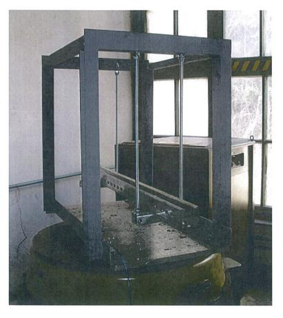
Fixing the testing assembly of cable channel type ATK-10-15 in testing apparatus and its "y" axis orientation thereto on vibrating stand
