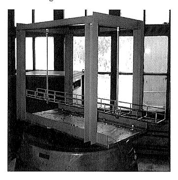
Fixing the testing assembly of cable ladder type A 20–FM–100–15 in testing apparatus and its "x" axis orientation thereto on vibrating stand
