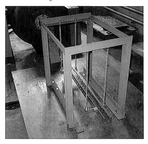
Fixing the testing assembly of cable channel type ATK-10-15 in testing apparatus and its "x" axis orientation thereto on vibrating stand
