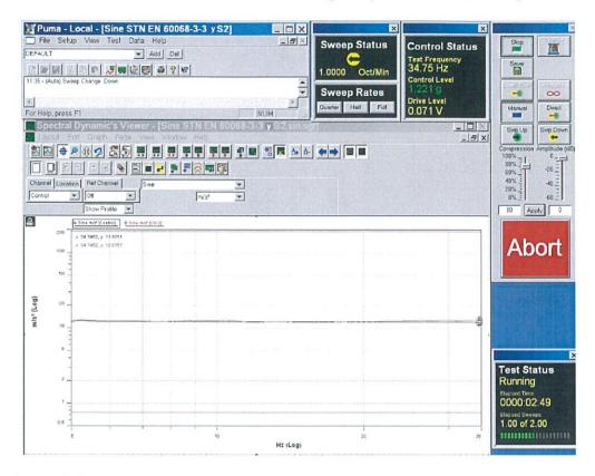
Recordings of signals from control sensor and sensor recording the vibration responses, cable ladder type A 20–FM–100–15, at test of resonant frequency assessment there in "x" axis.
