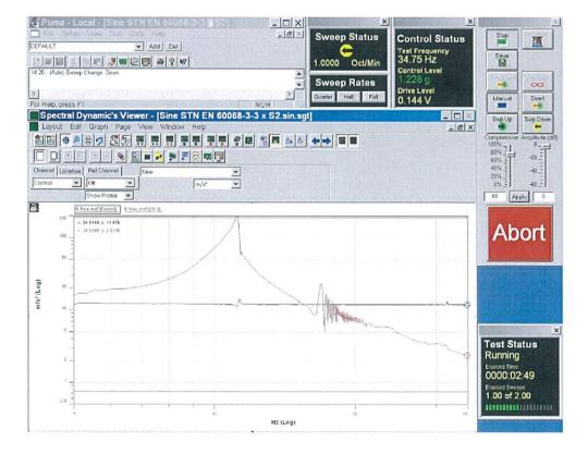
Recordings of signals from control sensor and sensor recording the vibration responses, cable trays type A 05–05A–15, at test of resonant frequency assessment there in "z" axis.
