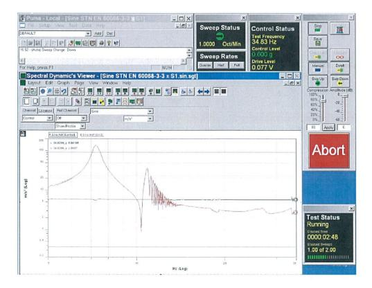
Recordings of signals from control sensor and sensor recording the vibration responses, cable channel type ATK-10-15, at test of seismic eligibility Level S2 there in "z" axis.
