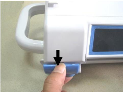
【Figure 60】 Pull the syringe grip out (pinch it and pull)
