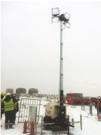
GENERAC® LED LAMPS 4x320 W high efficiency LED floodlights designed by Generac Tower Light.®
