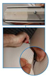
to do this, use a cross-head screwdriver. Gently move the screwdriver up and down along the length of the corner, until each of the 4 cross-head screws of the edge piece are located. Once the screw has been located, tighten it using the screwdriver.
