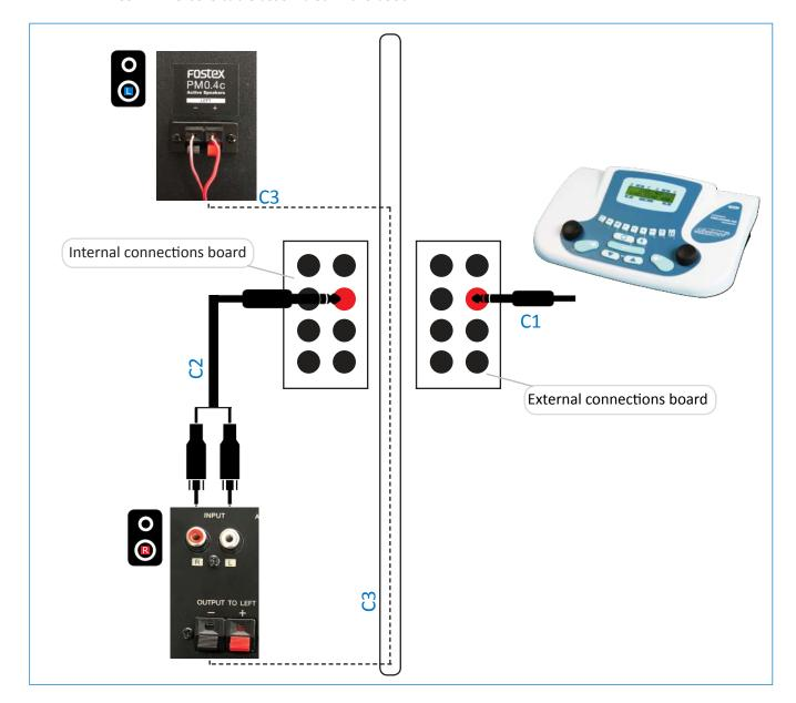
• Connecting a free-field system in audiometers that have two output connectors:
