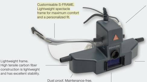
For any pupil size. Separate controls for convergence of optics and the angle of parallax guarantee fully illuminated stereo views in pupils up to 2 mm, as well as viewing in the periphery.
