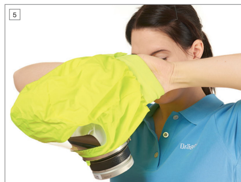
5 Widen the neck seal and pull the hood over your head. The inner head harness automatically adjusts to your head. Ensure that nose and chin sit comfortably in the half mask and that all hair is tucked into the hood.
