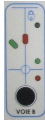
Deletion of logs is performed by the return of AC voltage or after 2 hours signalling. However, the information is retained for at least 3s after the fault has disappeared.
