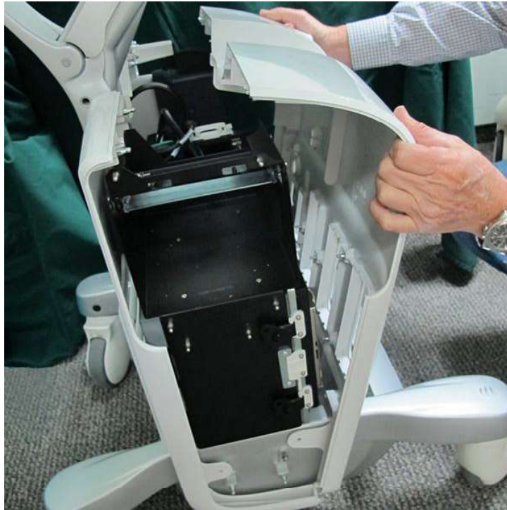
Figure 8-14 Removing the Front Cover
