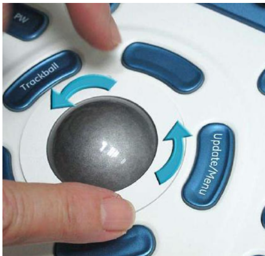
Figure 8-64 Removing the Mechanical Trackball Ring
