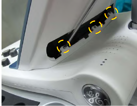
Figure 8-37 Removing the Rear Cover (Base) Securing Screws
