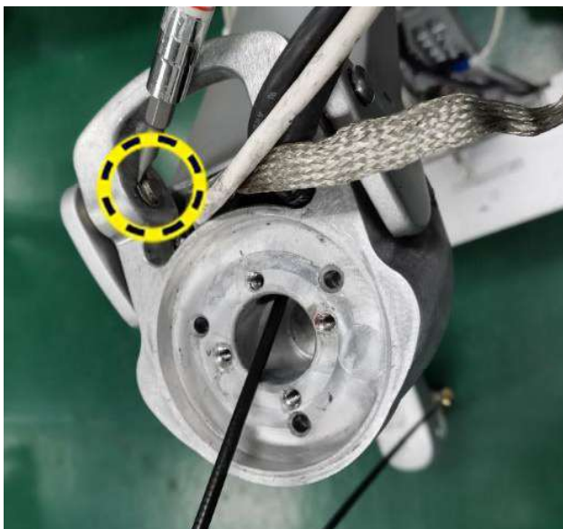
Figure 8-144 Ring Clips Securing Supporting Pins
