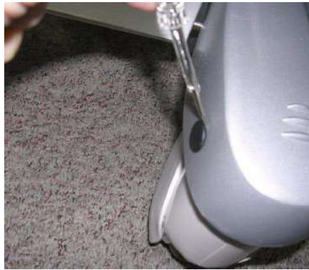
Figure 8-157 Removing the Screw Cap
