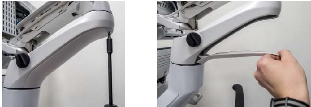
Figure 8-102 Remove the Lower Service Cover
