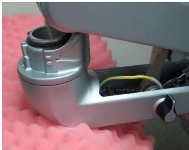
Figure 8-136 Protective Sponge Between Articulated Arm and System Handle
