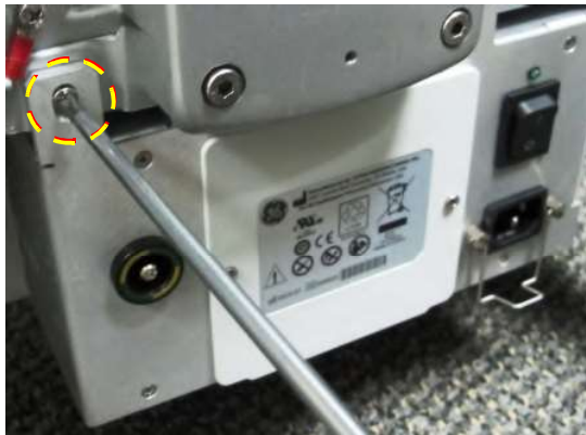
Figure 8-93 AC Box Supporting Screws
