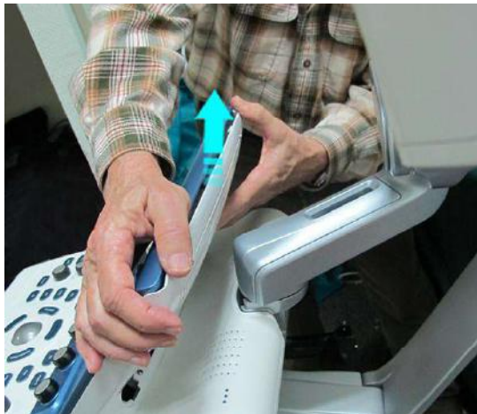
Figure 8-39 Removing the Touch Screen Rear Cover
