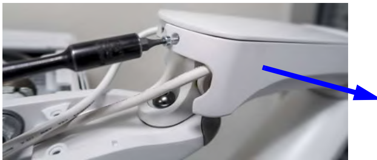
Figure 8-100 Remove the screw and the Upper Service Cover (one side illustrated)
