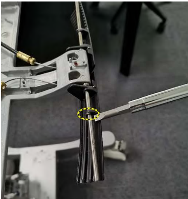
Figure 8-111 Remove spring clips
