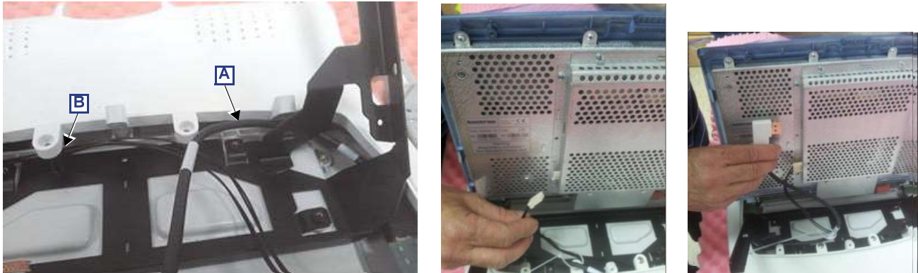
Figure 8-47 Routing and Connecting the Touch Screen Cables
