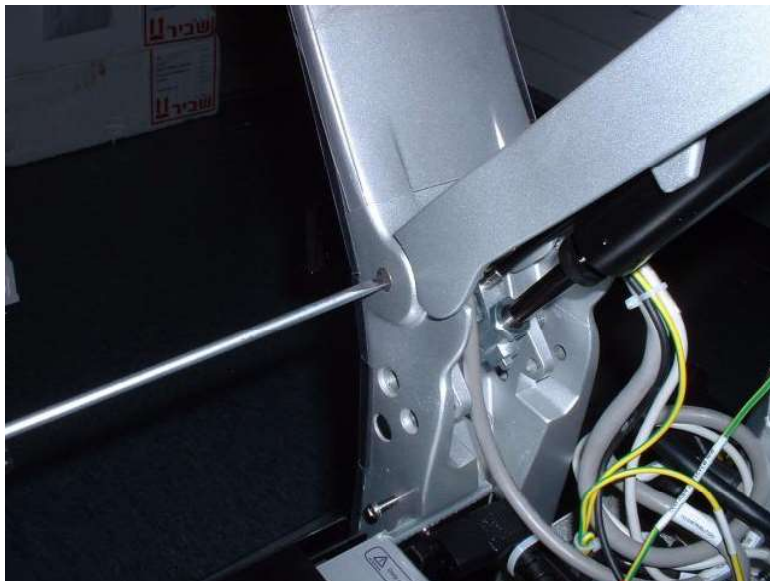
Figure 8-132 Tapping Out the Upper Arm Support Pin
