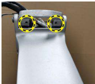
Figure 8-143 Locking Screws Securing the Joint Assembly Supporting Pins
