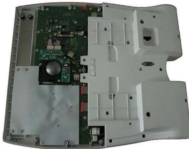
Figure 8-61 Operating Panel Keyboard Assembly with AN Keyboard/Bottom Cover Removed
