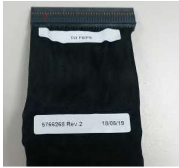
Figure 8-75 FEPS to MST cable
