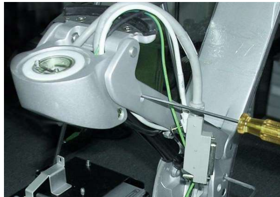
Figure 8-150 Supporting the Upper Gas Spring Bracket with a Screwdriver
