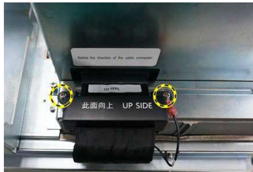
Figure 8-10. FEPS to CMST Cable
