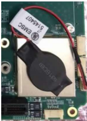
Figure 8-81 CMOS battery installed on BEP printed circuit board.
