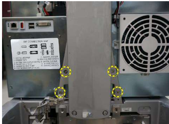
Figure 8-2. Install four screws at rear side
