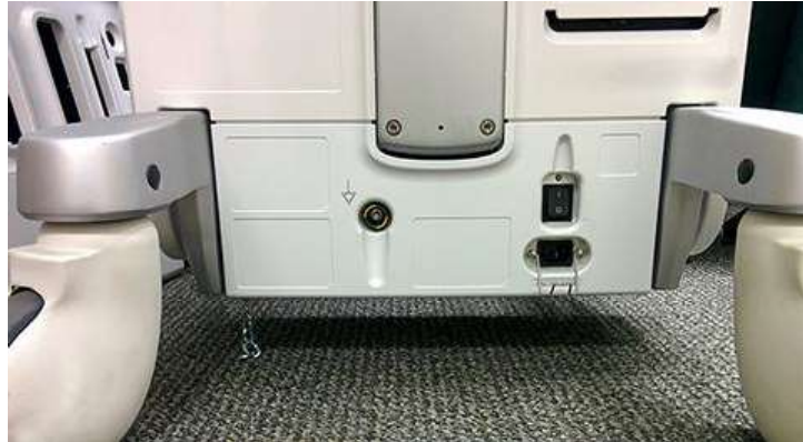
Figure 8-31 AC Distribution Box Cover Installed
