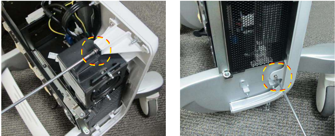
Figure 8-21 Left Rear Cover - Removing Securing Screws
