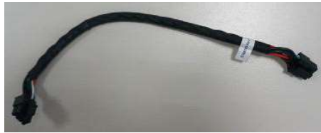
Figure 8-73 FEPS to BIF cable
