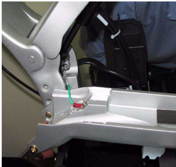
Figure 8-140 Removing the Lower Arm
