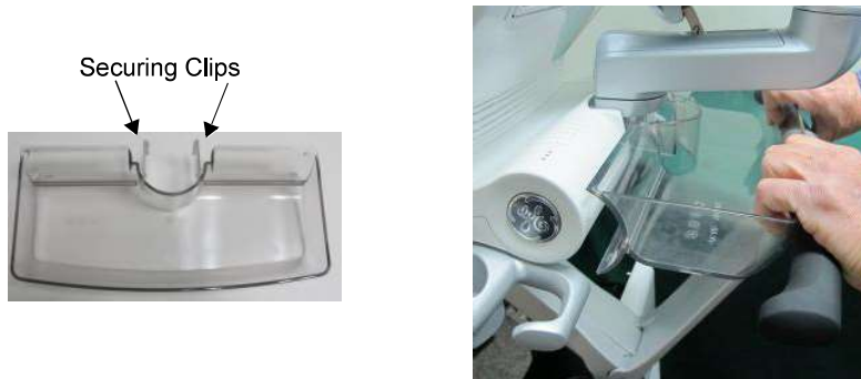
Figure 8-24 Removing the OPIO Basket
