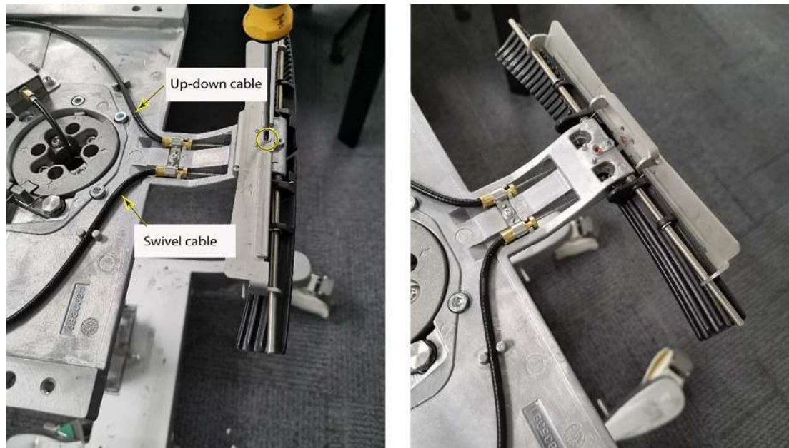
Figure 8-109 Protective Metal Plate Rotated 90 Degrees
