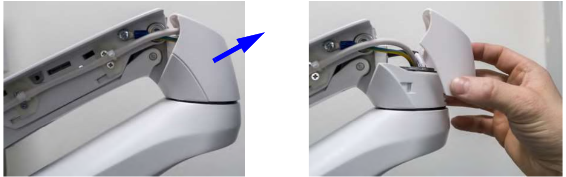
Figure 8-101 Remove the Vertical Service Cover
