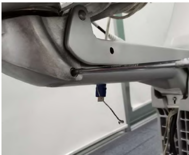
Figure 8-142 Unscrew the screw from one side
