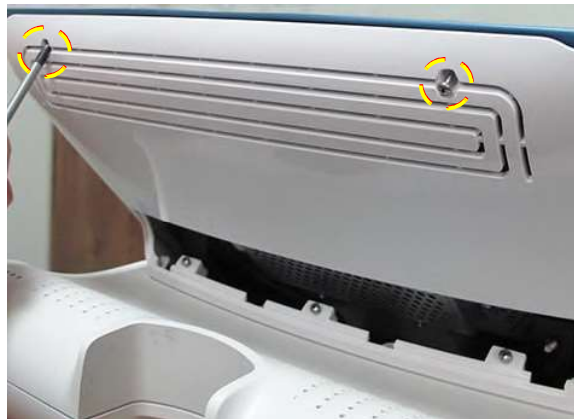
Figure 8-38 Removing the Rear Cover (Top) Securing Screws
