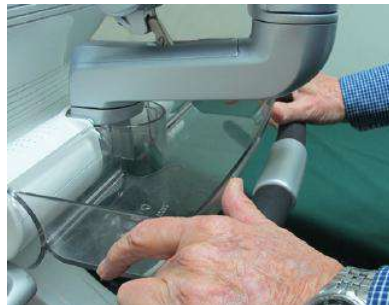
Figure 8-25 Installing the OPIO Basket
