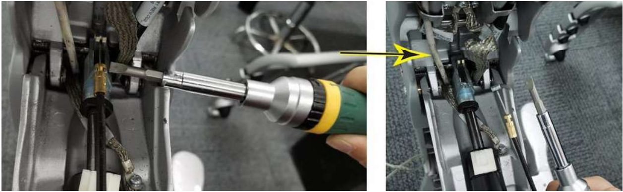
Figure 8-121 Remove up-down cable
