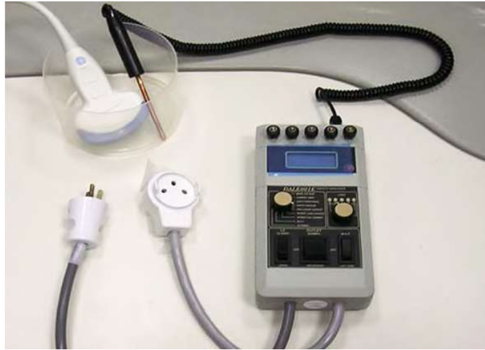
Figure 10-5 Test Set Up with Electrical Safety Analyzer
