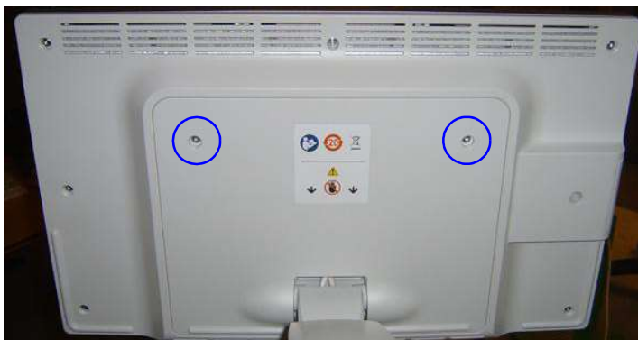
Figure 8-32 Monitor Rear Cover's fixing screws
