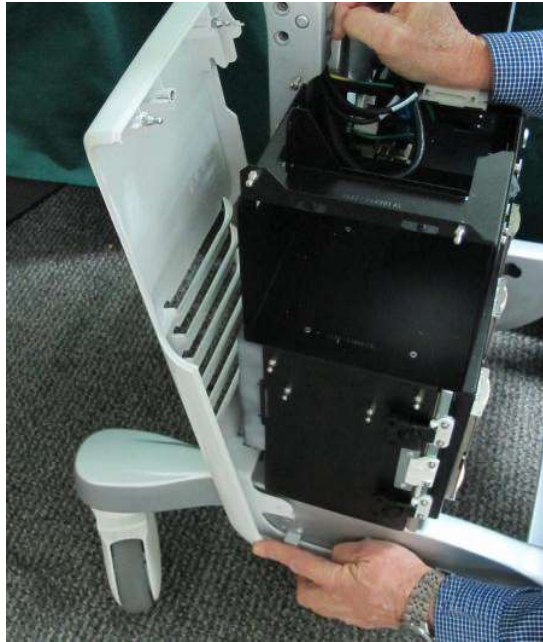
Figure 8-19 Removing the Right Rear Cover
