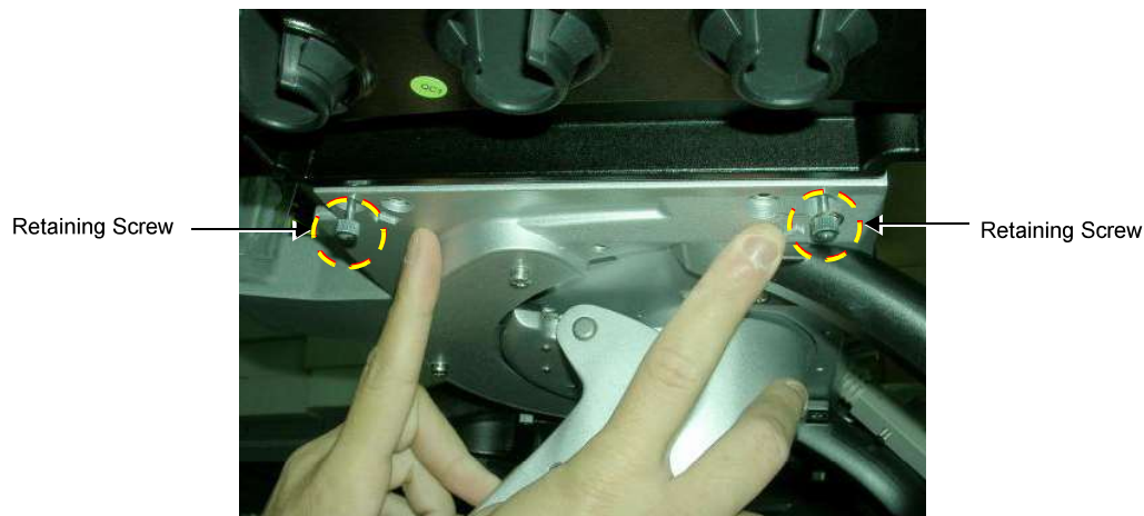
Figure 8-154 Probe Shelf - Viewed from Below indicating Retaining Screws
