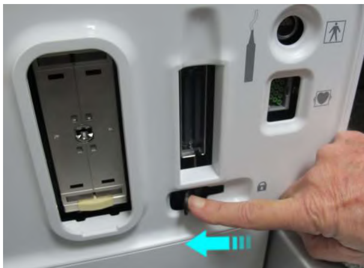
Figure 8-11 RS Probe Connector Lock - OPEN
