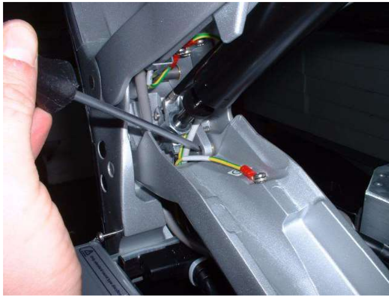
Figure 8-139 Removing Securing Pin and Disconnecting Ground Lead
