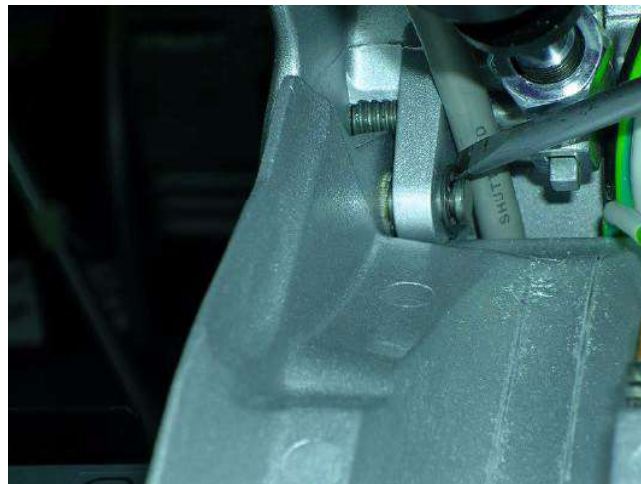
Figure 8-138 Removing Left Securing Clip from Securing Pin
