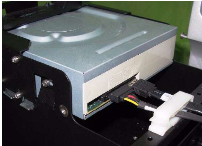
Figure 8-215 Cables Connected at Rear of DVD/CD-RW Drive
