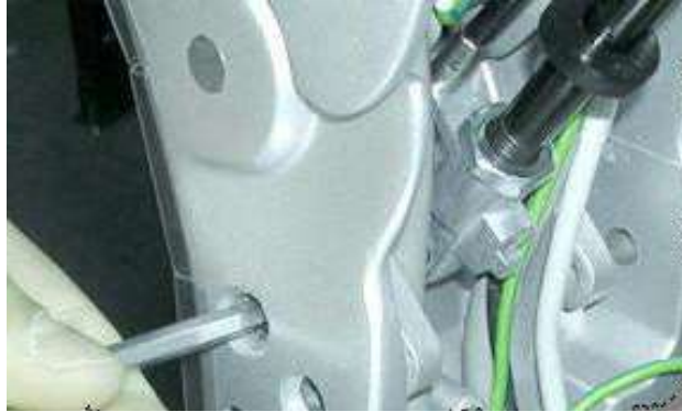
Figure 8-148 Releasing the Securing Screws on Either Side of the Support Arm
