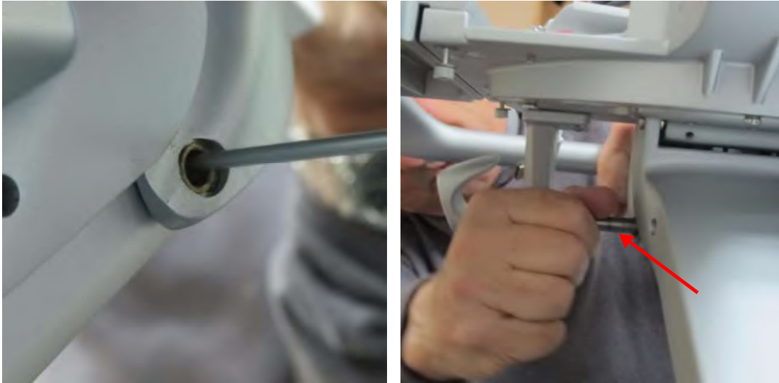
Figure 8-135 Remove Securing Pin
