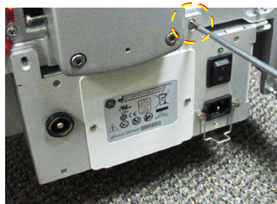
Figure 8-93 AC Box Supporting Screws
