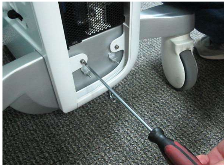
Figure 8-13 Removing Screw from Front Cover Securing Tab
