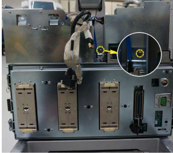
Figure 8-1. Install screw on front side
