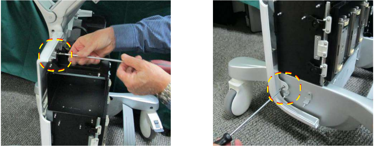
Figure 8-17 Right Rear Cover - Removing Securing Screws
