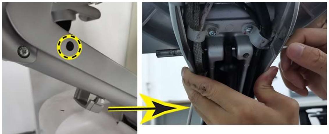
Figure 8-120 Remove screw covers and push out pins
