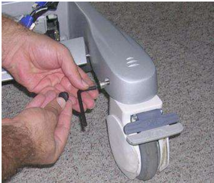
Figure 8-158 Removing the Securing Screw
