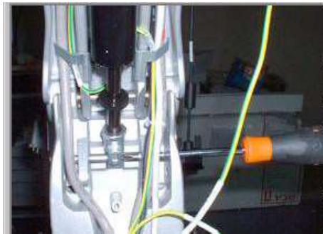
Figure 8-149 Tapping out the Lower Support Pin using a Punch
