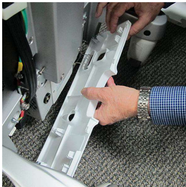
Figure 8-30 Removing the AC Distribution Box Cover
