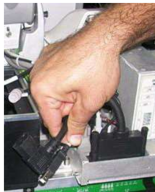
Figure 8-218 Cables Disconnected from Rear of Black and White Printer
