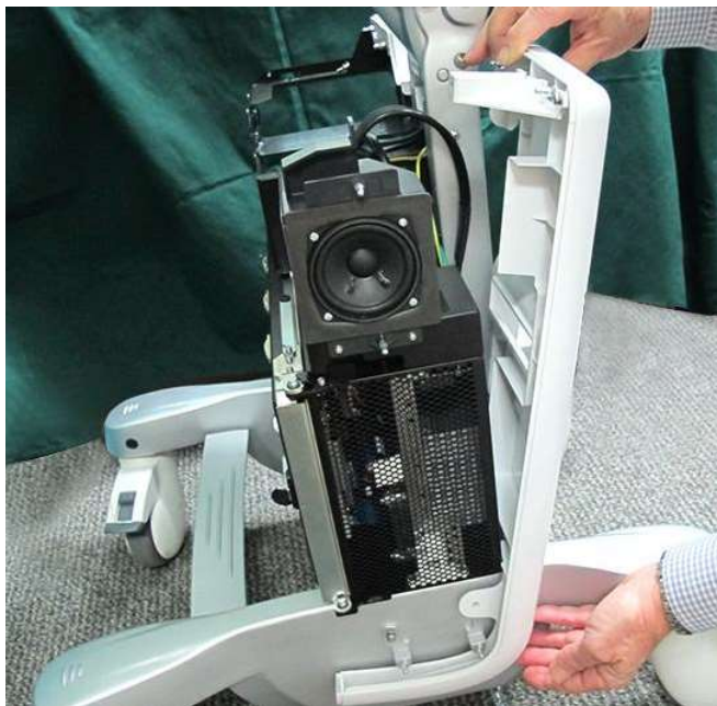
Figure 8-23 Removing the Left Rear Cover
