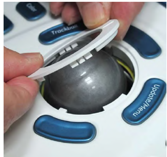
Figure 8-64 Removing the Mechanical Trackball Ring
