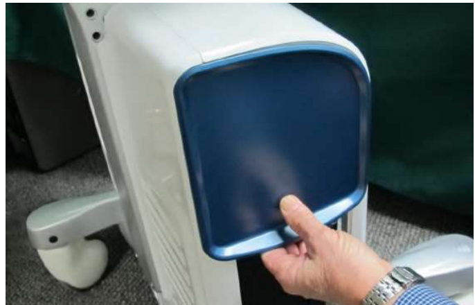
Figure 8-8 Removing the Blank Cover
