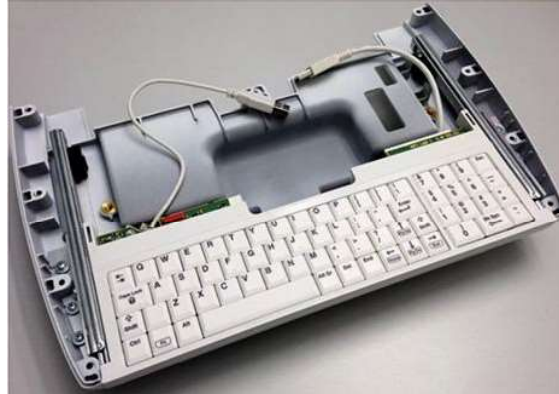
Figure 8-58 Alphanumeric Keyboard/OPIO Bottom Cover Assembly
