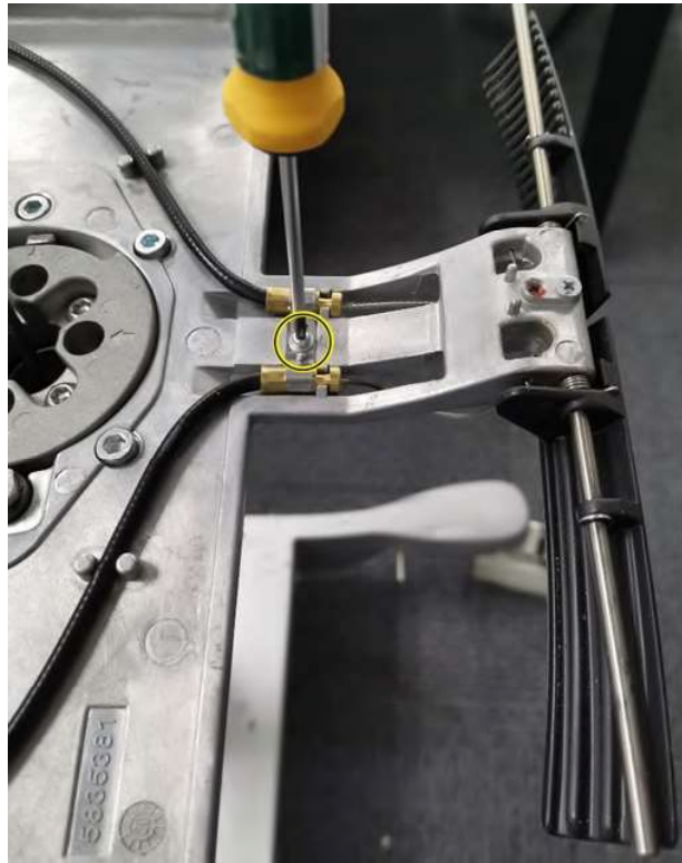
Figure 8-124 Unscrew cable clip
