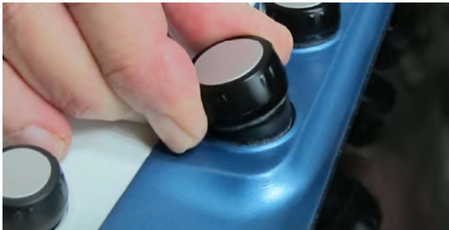
Figure 8-68 Removing a Rotary Knob
