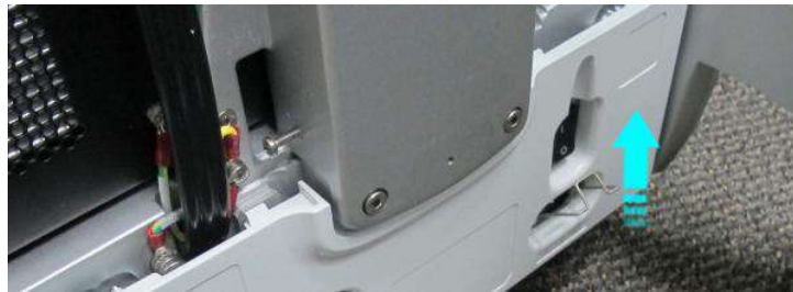
Figure 8-29 Removing the AC Distribution Box Cover
