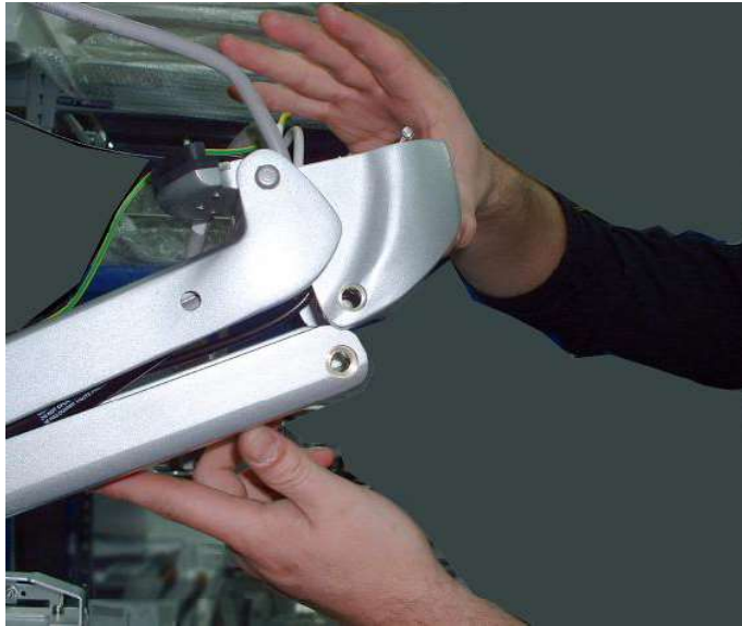
Figure 8-141 Raising Lower Arm to Reconnect with Upper Arm (Console not shown)
