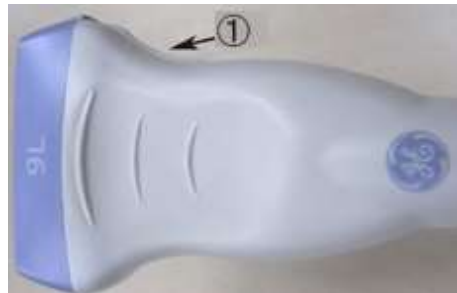
Figure 11-1. Orientation Marking on Probe (Example)
