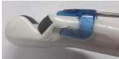
Figure 11-32. Align the biopsy guide
