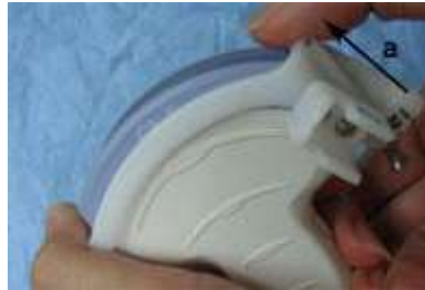
Figure 11-18. Remove the biopsy guide
