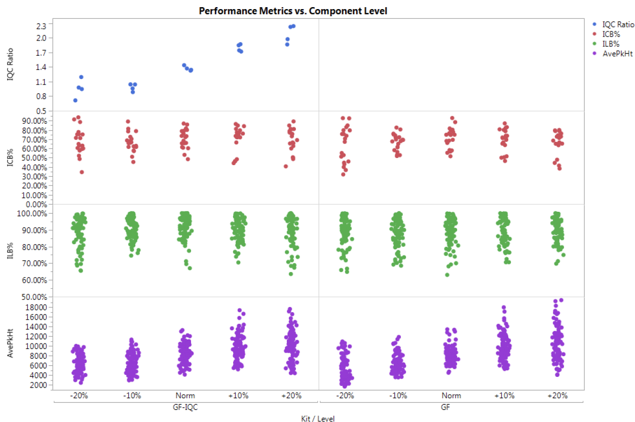
Figure 68 Master mix amount variation for GlobalFiler™ IQC (left) and GlobalFiler™ (right) kits. Input is \pm 20\% of standard 7.5 \mu\text{L} input per 25 \mu\text{L} reaction (with standard primer mix amount) with 1.0 ng of Control DNA 007.
