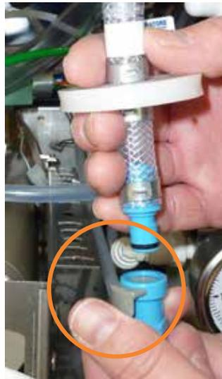
**Figure 3 Pressing Quick Connect Button**
