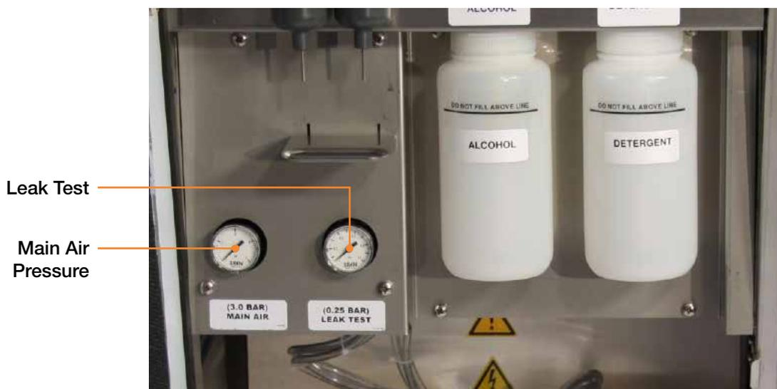
**Figure 1 Air Pressure Controls**
