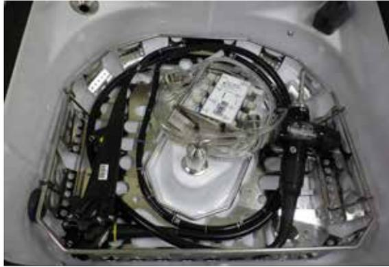
**Figure 16 Fit the Light Guide Tube in Basin**
