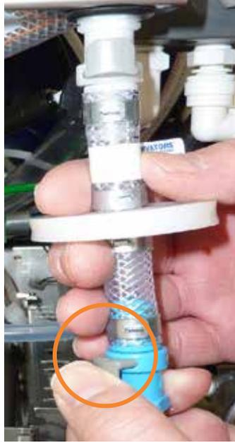
**Figure 2 Quick Connect Fitting**
