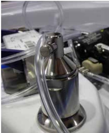
**Figure 19 Sprayer Must Turn Freely**
