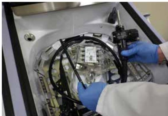
**Figure 15 Set the Insertion Tube in Basin**
