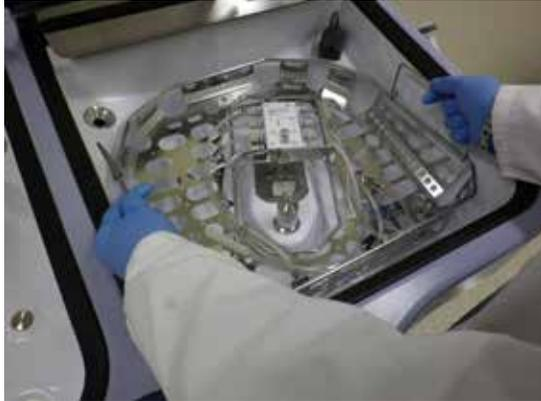
**Figure 11 Fitting the Connector Block**
