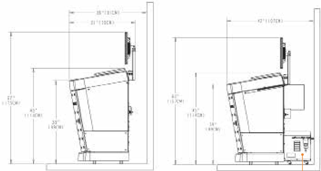
Figure 2 Side Dimensions and Clearance
