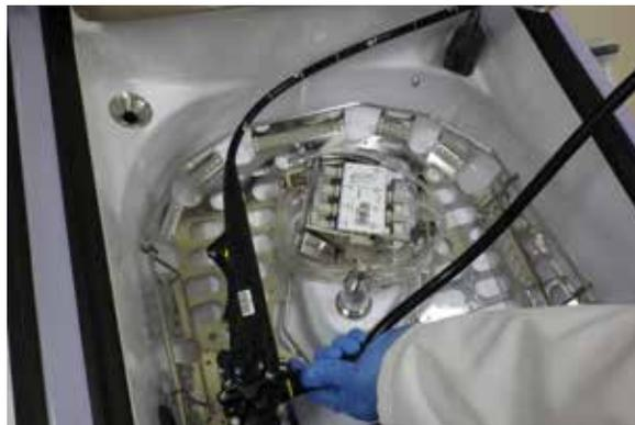
**Figure 14 Place Control Housing in Basin**
