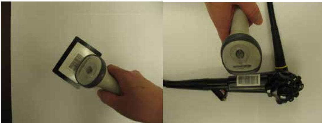
**Figure 11 Barcode Reader for Operator Login and Endoscope ID**
