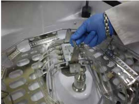
**Figure 12 Press Block Over the Manifold**
