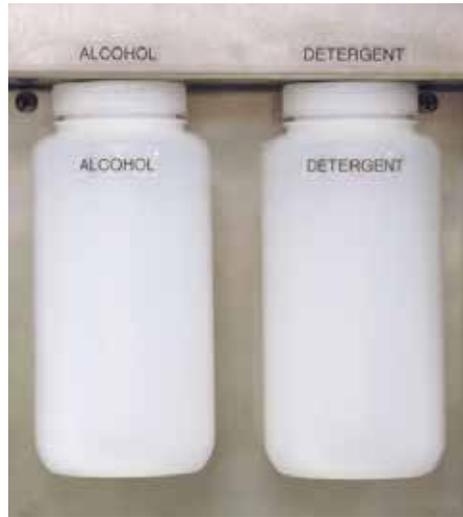
**Figure 25 Alcohol and Detergent Reservoirs**
