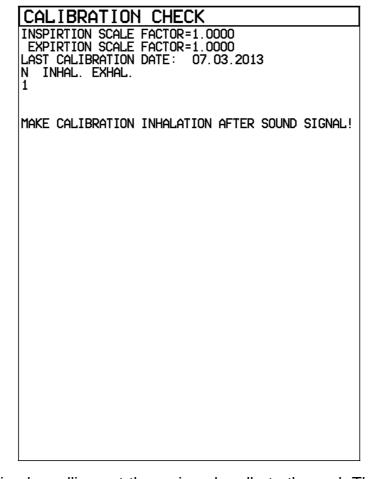
Make inspiration by pulling out the syringe handle to the end. The inspiration should be performed smoothly without jerks within 1-2 seconds time. Calibration result will appear on display and the message "MAKE A CALIBRATED INHALATION AFTER A SOUND SIGNAL!" will change into "MAKE A CALIBRATED EXHALATION AFTER A SOUND SIGNAL!"
