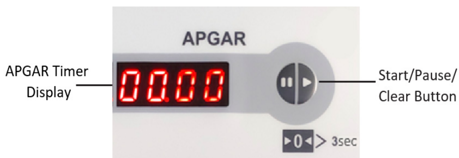
Figure 3-8. APGAR timer interface
