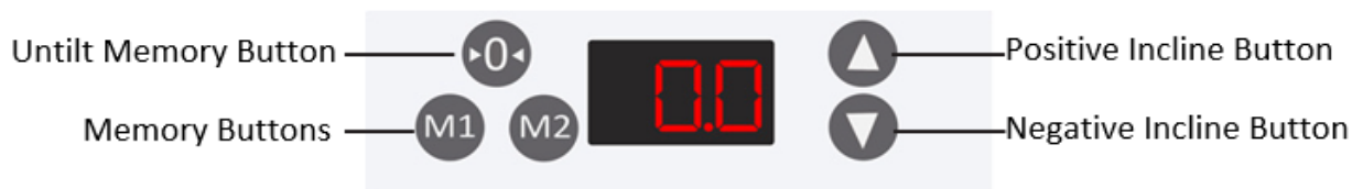
Figure 4-2. Electronic trendelenburg user panel
