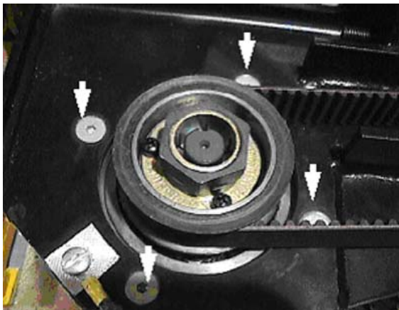
Figure 13. Removing the four (4) hex screws will release motor.
