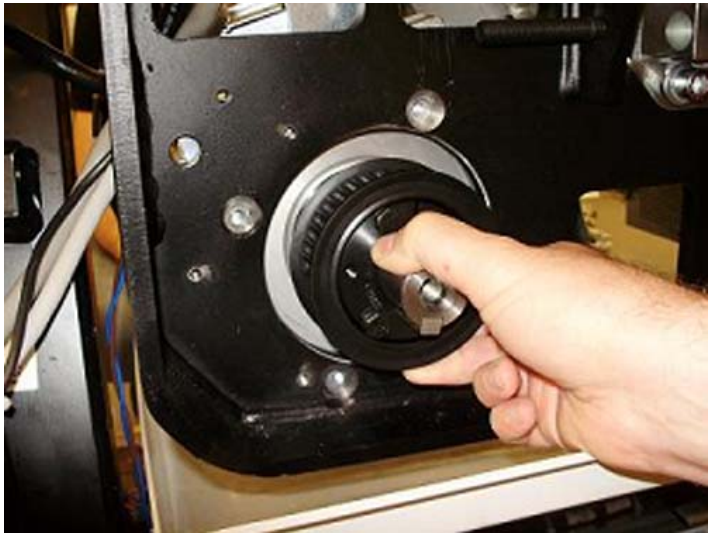
Figure 16. Pull back on motor hub to hold in place before bolting to frame.
