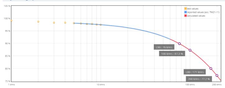
LxB50 results according to LM-80 and TM-21-11 procedures and norms.
