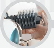
VITEK 2 Compact: Cards inoculated inside instrument and manually transferred from filling door to loading door for processing
