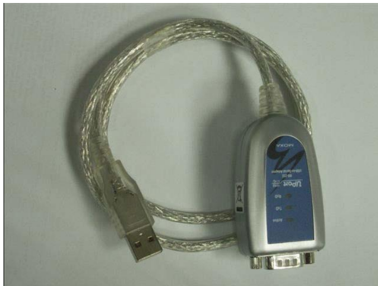
Figure 69 - The MOXA Adapter
