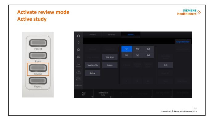
To activate the review mode during an active examination, press the **Review** key on the Control Panel.
