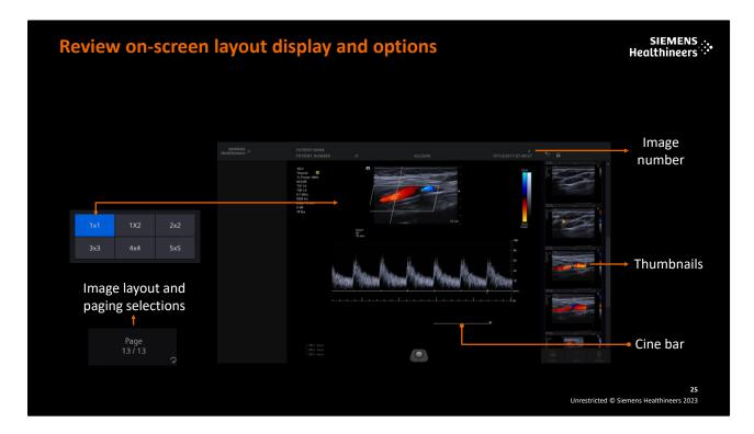
When review is activated, the system displays all images and clips saved with the study in the thumbnail panel and displays at least one image or clip on the review screen.
