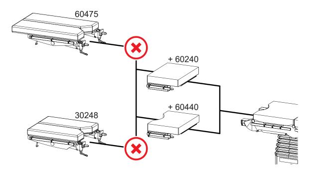
Figure 12. Non-motorized leg sections with SWL 160 kg
