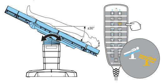
For full Trendelenburg adjustment range, the table top must be higher than the first 130 mm of the height adjustment range. Tilt must be adjusted to horizontal position. Otherwise the table top will rise automatically to the minimum height to enable the full range of adjustment when you keep the Trendelenburg adjustment button pressed. This is indicated by a continuous beeping sound.
