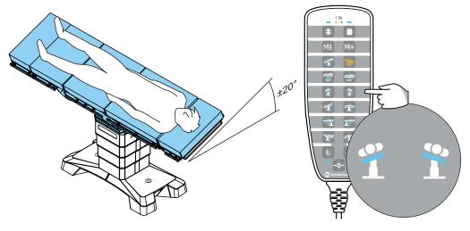
The tilt range is limited if the table top is within the first 130 mm of the height adjustment range and if the Trendelenburg adjustment angle is steep.
