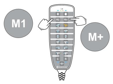
To use the preset position, keep the **M1** memory position button pressed until the table reaches the saved position.
