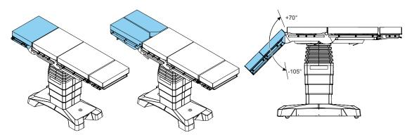
Divided leg sections and undivided one-piece leg sections are adjusted in the same way.
