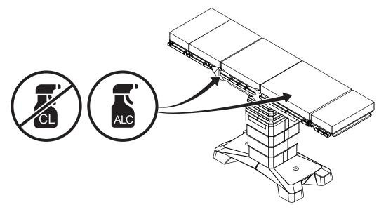
Gently rinse or wipe with a damp cloth to remove disinfectant residues from stainless steel parts, such as accessory rails, seat joints and joint cover plates, latches, and table top screw heads.
