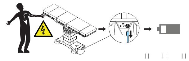
Disconnect the mains cable and use the operating table in battery mode.
