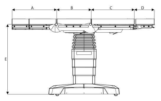
Table 19. Table top dimensions with motorized leg section
