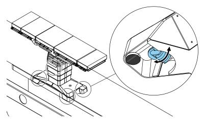
3. Extend and retract all table adjustments and check the -0- positioning function.
