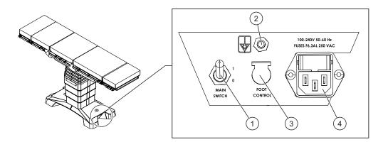
The main switch is located on the table base on the head section side of the table.
