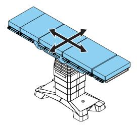
6. Ensure that accessory rails are properly mounted and not worn.
