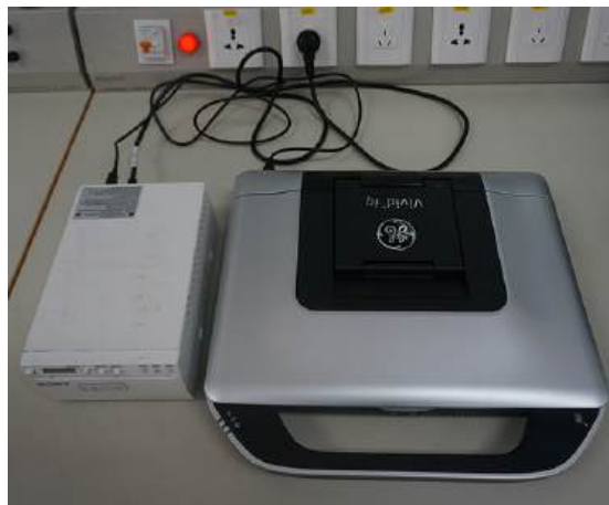
Figure 3-4. UP-D898 MD connection
