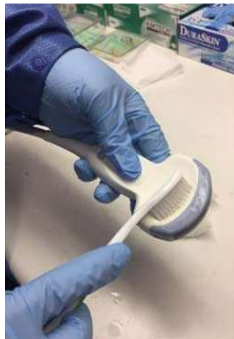
Figure 11-6. Cleaning the probe using a brush
