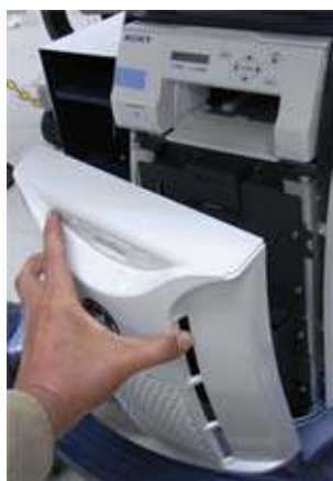
Figure 12-9. Remove the front cover
