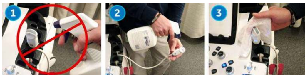
Figure 12-8. DO NOT Spray a Probe While in its Holder
