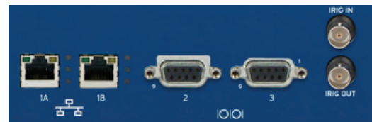
Figure 3 Rear-Panel Communications and IRIG-B Ports
