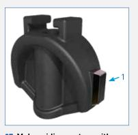
07: Male guiding system with composite sliding skate (1) reduces the wear of the wedge against the body, allowing a smooth functionality and a longer life time of the valve. Furthermore, the increased thickness of the elastomer at the sealing areas improves product resilience to the usual small impurities encountered in networks.
