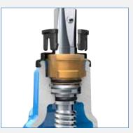
05: The three locking tabs for bayonet system as well as clamping ring prevent self-dismantling, caused mainly by over-torques and vibrations, to avoid risk of leakage and also prevent incidents and ensures the safety of all personnel on site.
