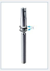
04: Stem and collar made in one piece in stainless steel for better resistance to axial load and to withstand higher operating torques. Washers with PTFE coating (1) placed above and under the collar allow to reduce friction torque and protect coating inside the Bonnet.
