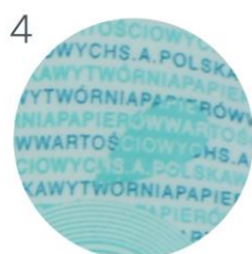
4 Positive and negative micro-printing with case modulation
