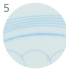
5 Microtext partially overlapping photo area
