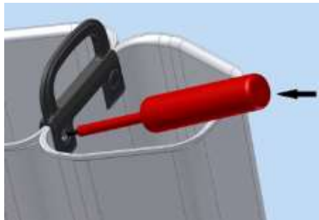
Fig. 62: Pushing the opposite rivet out
