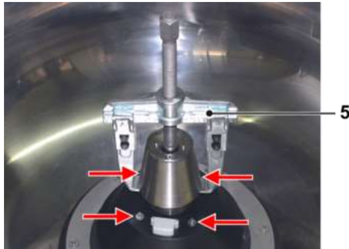
Fig. 16: Position of the screws of the cover collar (partly hidden)
