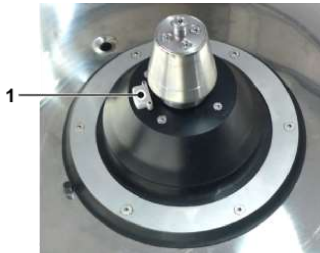
Fig. 38: Rotor identification system in the rotor chamber
