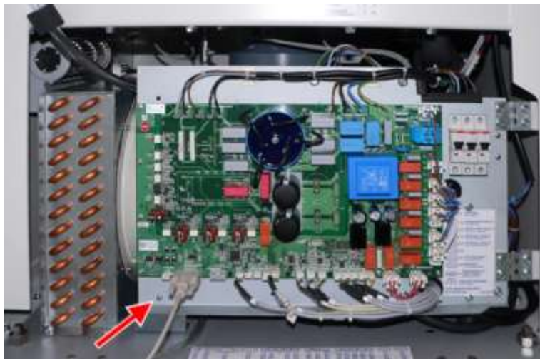
Fig. 30: Position of the screw for loosening the power module
