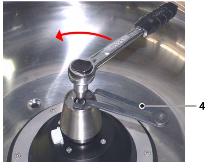
Fig. 15: Loosening the screw of the cone
