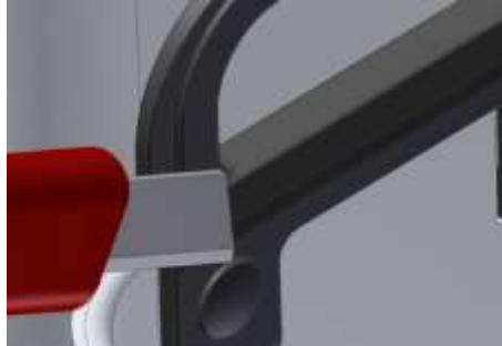
Fig. 61: Cutting the rivet head off
