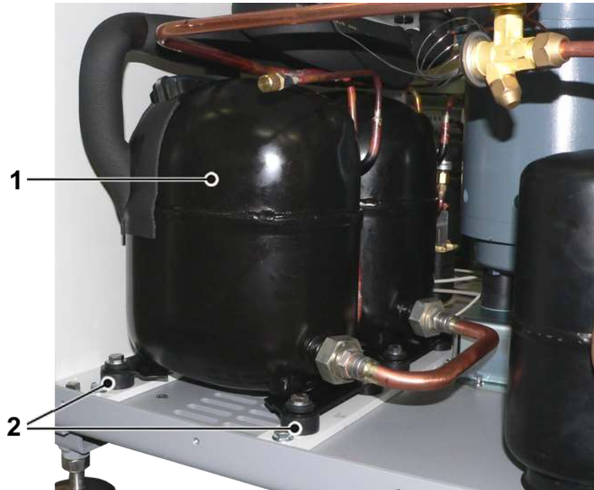
Fig. 26: Compressor, view from the back
