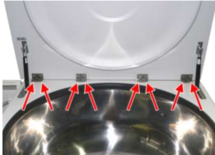
Fig. 6: Position of the hinge screws of the centrifuge
