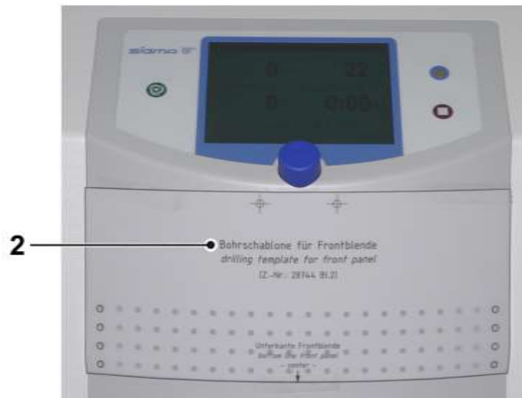
Fig. 56: Front panel with the drilling template
