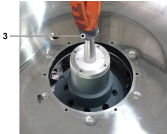
Fig. 21: Drive unit with an eye bolt and round sling
