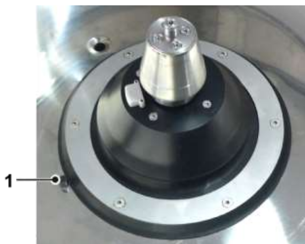
Fig. 36: Temperature sensor in the rotor chamber
