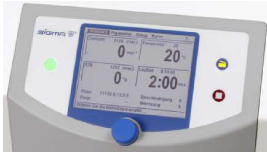
Fig. 44: Control panel of the Zent7 control system, old variant
