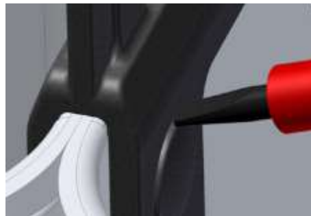
Fig. 59: Positioning the tool between the rivet and handle
