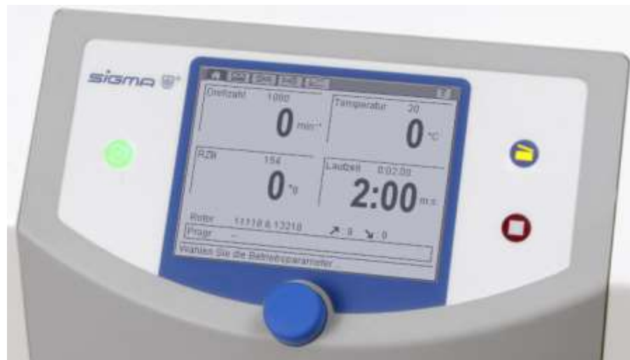
Fig. 45: Control panel of the Zent7 control system, new variant
