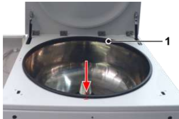
Fig. 9: Position of the seam of the lid gasket
