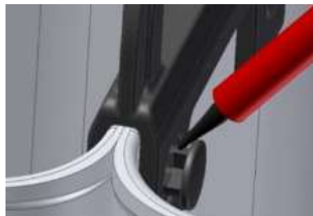
Fig. 60: Pushing the tool further in behind the loosened rivet
