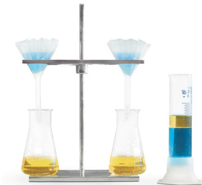
Grade 480 is impregnated with stabilized silicon, thus rendering it hydrophobic: It retains water, but allows solvents to flow through. The flow stops automatically when the entire solvent has passed through. In many applications, this phase separator paper eliminates the need to use separating funnels.
