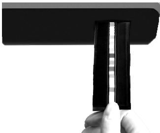
**Note:** In order to avoid contamination of the strip holder and/or the optical sensor, make sure that the strip holder is fully extended and at a standstill before placing or removing a urine strip from the strip holder.
