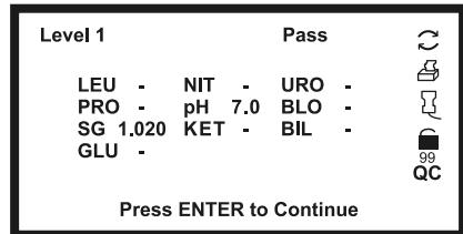
If any parameter is out of range, it will be highlighted and marked with a “\*”.
