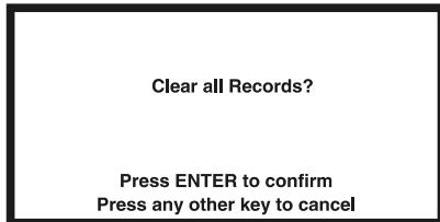
Press **ENTER** to delete all records. A prompt will appear. Once records are deleted they cannot be recovered. The **Test Number** will reset to 000001, 100001 or 200001 depending on the Test Mode. Press any other key to cancel. The screen will return to the **Database Menu**.
