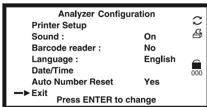
Press **▲** or **▼** to move **→** to make changes. After all changes are made, select **EXIT** and press **ENTER** to save changes and return to the **Main Menu**. If **User Login** is enabled and **Operator ID** is 11 through 20, this **Menu** cannot be changed.
