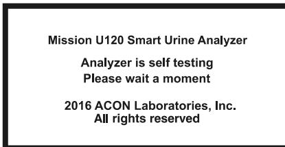
Turn the Power Switch on. If the Self-Test passes, the Initial Screen will be shown.
