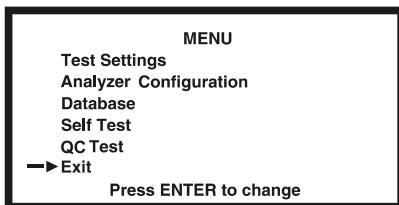
Select options by pressing **▲** or **▼** until the Selection Arrow (→) is next to the option. Press **ENTER** to show the options in a new screen or cycle through the settings below. Select **Exit** and press **ENTER** to return to the Initial Screen.
