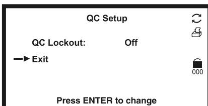
**On** enables the QC lockout function. The **QC** symbol is displayed. QC Lockout timing can be set for **Every 8 Hours**, **Daily**, **Weekly** or **Monthly**.
