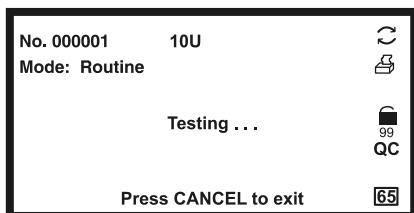
The countdown clock is displayed on the bottom right of the screen. The clock will start to count down from **65**. The operator has 3 seconds before the triple beep sounds to immerse the strip into the urine.
