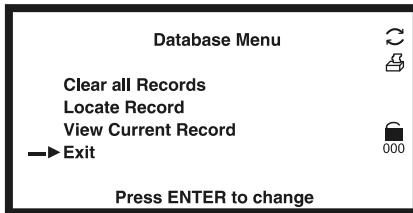
Press **▲** or **▼** to move **→** to enter each screen and make changes. After all changes are made press **ENTER** to save changes and return to the **Main Menu**.
