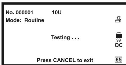
The countdown clock is displayed on the bottom right. The clock will start to count down from **65**. The operator has 3 seconds before the triple beep sounds to immerse the strip into the urine.
