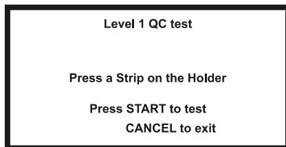
The analyzer will run a Level 1 QC test first. Refer to the Strip Test section for details on testing.
