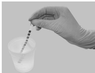
Run the edge of the strip against the rim of the urine specimen container to remove excess urine. Hold the strip in a horizontal position. Bring the edge of the strip into contact with an absorbent material (e.g. a paper towel). This prevents mixing chemicals from adjacent reagent areas.
