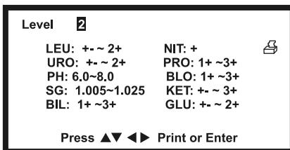
Press **▲** or **▼** to change the highlighted digit. Press **◀** or **▶** to move to the digit to be changed. Press **▲** or **▼** to increase or decrease the value. Change each of the analyte QC values in this manner until the desired values are shown. Press **ENTER** to save the changes and exit the screen. Press **PRINT** to print the current values.
