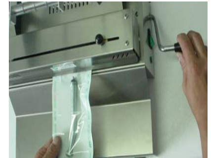
Graph 8: Sealing Schematic of Packing Bag with Substance to be Sterilized
