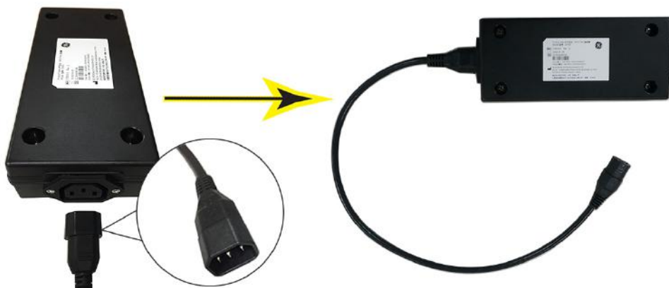
Figure 3-50. Insert the cable into the EMI filter output side
