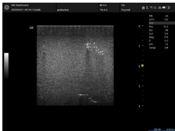
Figure 3-63. Abnormal image acquired with a deficient 12L-RS probe that has distributed defect elements
