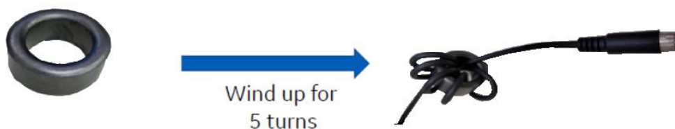
Figure 3-53. Wind up the Ferrite core assy to the S-video cable
