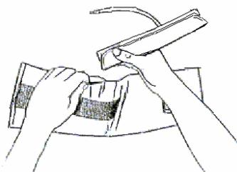
Fig. 8-3 Replacing Rubber Bags in the Cuff
