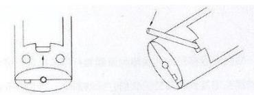
Fig. 7-2 Removing the Battery Cover
