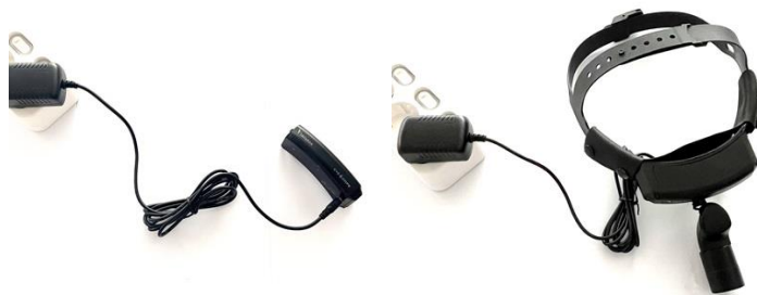
Fig. 3.3 Two way of charging the battery pack
