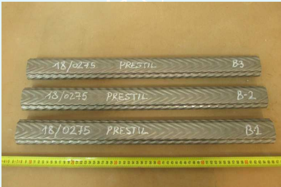
Photo of ribbed, press-bent sections
